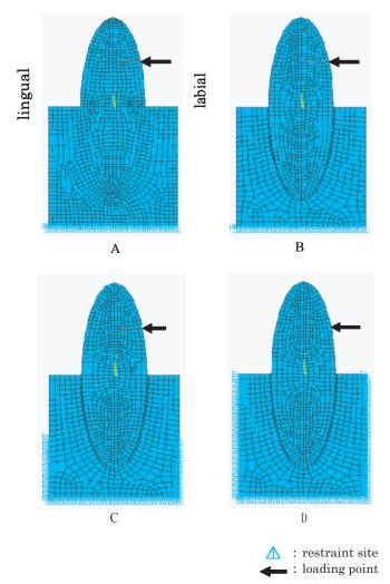
**Fig. (1).** 2-D FE models of mandibular central incisors under various conditions.
