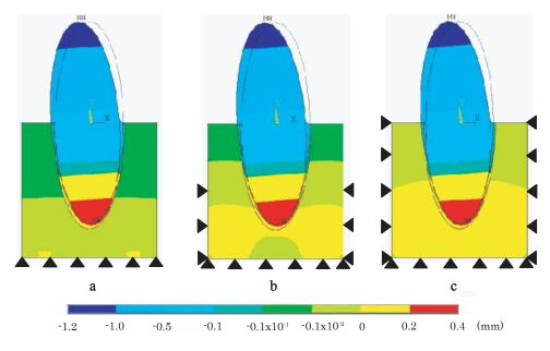
Fig. (5). Difference of displacement on PDL models with various restraint conditions.a: Model B (base restrained), b: Model C (base + side 1/2 restrained), c: Model D (a whole restrained).
