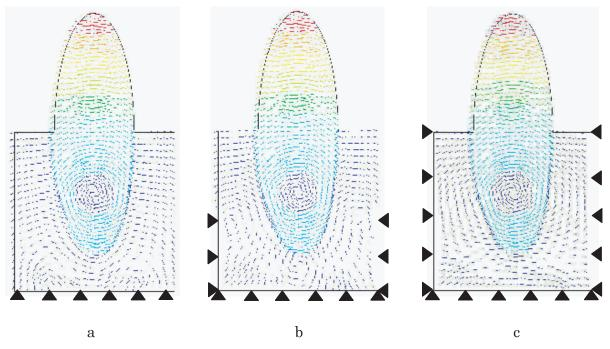
**Fig. (6).** Difference of vector indication of displacement on PDL models with various restraint conditions. **a:** Model B (base restrained), **b:** Model C (base + side 1/2 restrained), **c:** Model D (a whole restrained).
