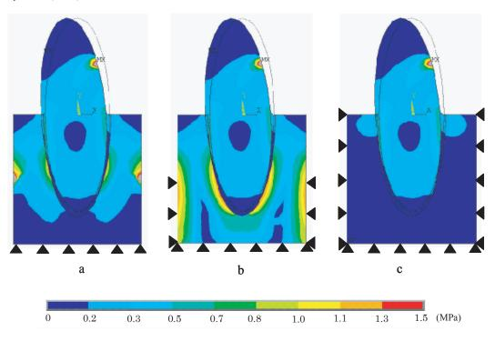
Fig. (4). Difference of equivalent (Von Mises) stress distribution on PDL models with various restraint conditions.
