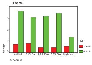
Fig. (1). Leakage in enamel after 24 hours and 6 months storage.
