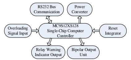
Fig. (2). Lower machine control system structure.
