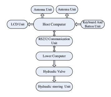
Fig. (1). The whole control structure.
