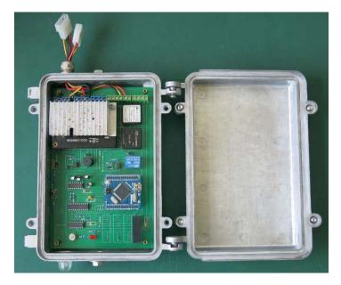
Fig. (11). The developed controller.
