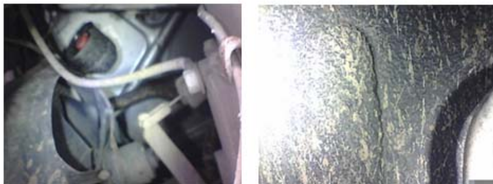
Fig. (9). Image captured by the chassis inspection robot.
