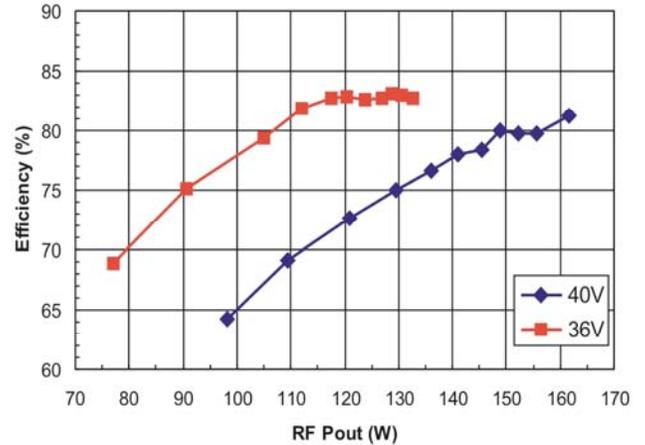
Fig. (5). Power supply efficiency for two input operating voltages for the entire circuit.
