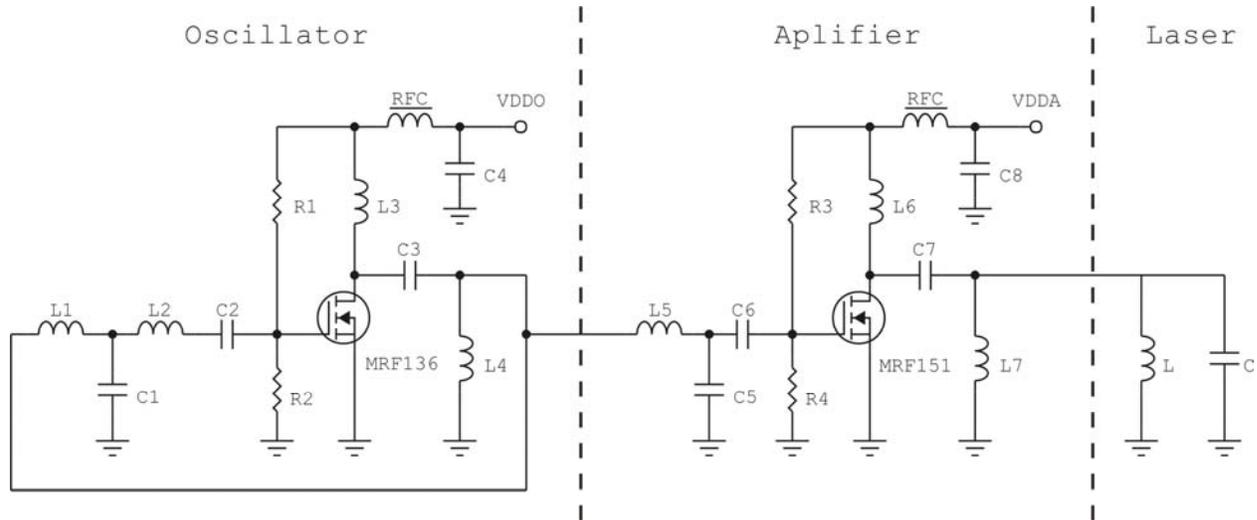
Fig. (1). Two stage RF excitation circuit diagram.
