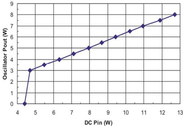
Fig. (2). Behavior for the oscillator output power in terms of the DC input power.
