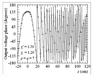
Fig. (5). Phase of the probe voltage on the generatrix at  $\varphi = 0^{\circ}$ . Solid line: measured. Crosses: interpolated.
