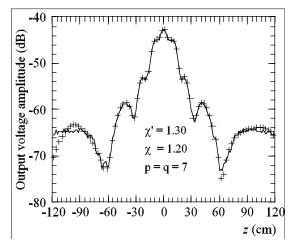
Fig. (4). Amplitude of the probe voltage on the generatrix at  $\varphi = 30^{\circ}$ . Solid line: measured. Crosses: interpolated.
