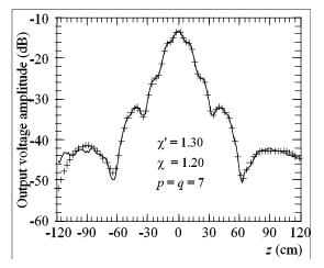
**Fig. (3).** Amplitude of the probe voltage on the generatrix at  $\varphi = 0^\circ$ . Solid line: measured. Crosses: interpolated.
