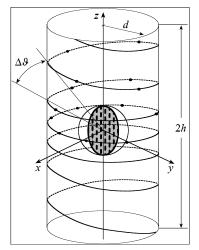
Fig. (1). Helicoidal scanning.
