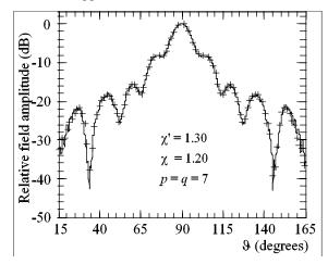
Fig. (6). E-plane pattern. Solid line: reference. Crosses: reconstructed from NF data acquired *via* helicoidal scanning.
