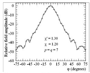
**Fig. (7).** H-plane pattern. Solid line: reference. Crosses: reconstructed from NF data acquired *via* helicoidal scanning.
