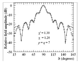
Fig. (8). E-plane pattern. Solid line: direct FF measurements. Crosses: reconstructed from NF data acquired *via* helicoidal scanning.
