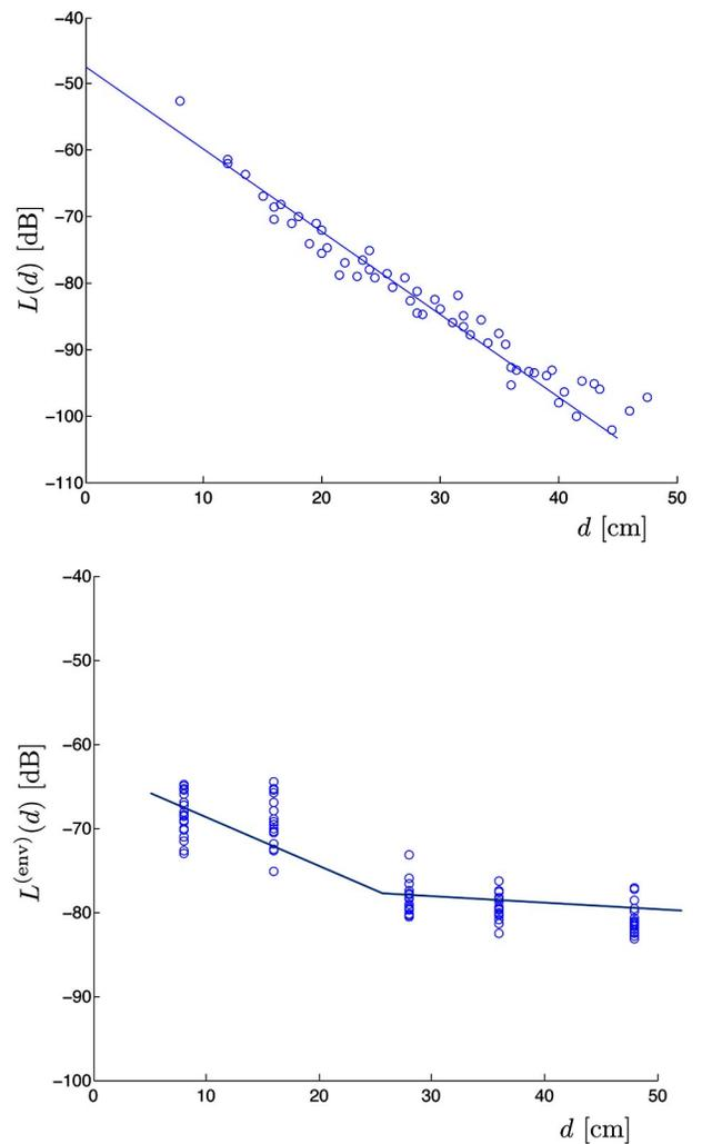
Fig. (2). On-body propagation loss as a function of the distance: experimental results (circles) and linear interpolation (solid line).
