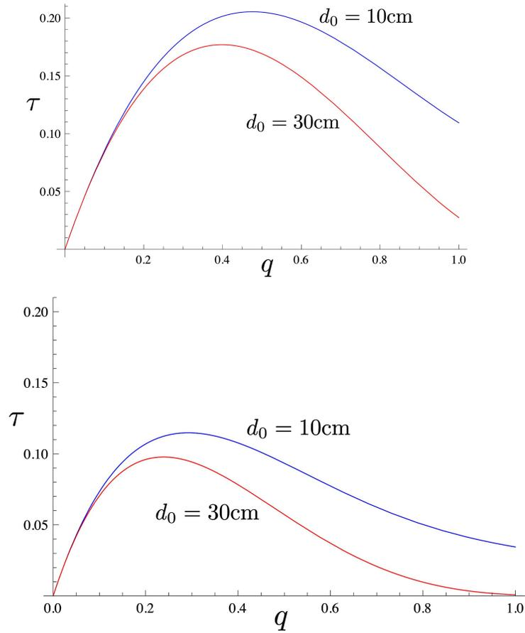
**Fig. (6).** Link throughput, as a function of  $q$ , (a) in a scenario with 2 close sensors and 2 far sensors and (b) in a scenario with 4 close sensors and 4 far sensors. In all cases,  $\theta = 5$  dB and  $\sigma = 8$  dB.
