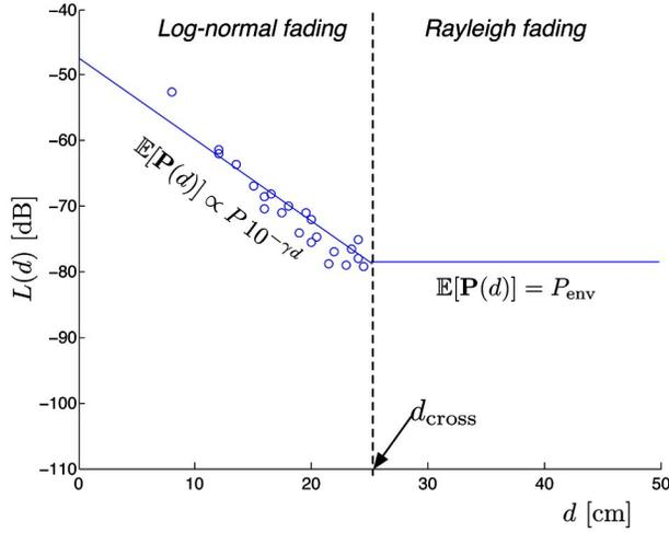
Fig. (3). Generic propagation model (on-body and environment reflection superimposed)
