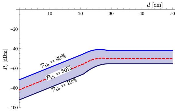
Fig. (4). Minimum transmit power as a function of the distance. The dashed region is the operational region of a BAN.
