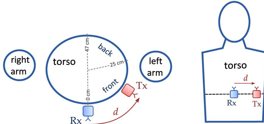
Fig. (1). Possible positions of a transmitter-receiver pair in a BAN.
