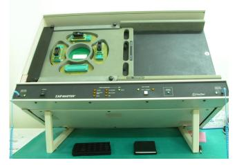
Fig. (1). An ESD test machine (KeyTek Zapmster 7/4).
