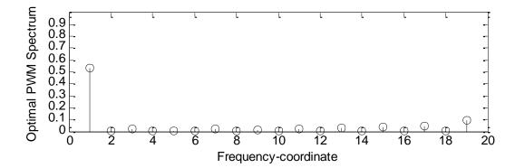
Fig. (5). The sinusoidal gratings's spectrum based on Optimal PWM.
