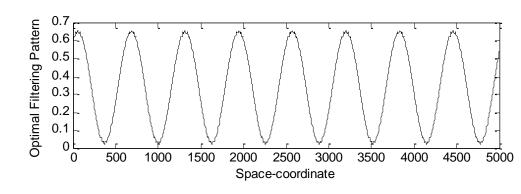
Fig. (7). Optimal PWM pattern after filtering.
