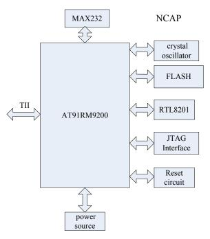
Fig. (3). NCAP principle block diagram.
