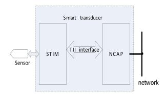
Fig. (2). Smart transducer structure.
