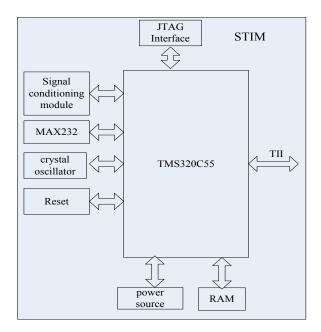
Fig. (6). STIM principle block diagram.
