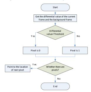
Fig. (2). The flowchart of background subtraction.
