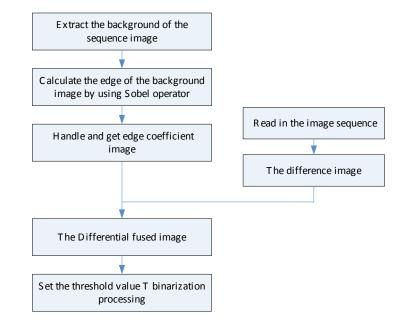
Fig. (1). The flow chart of adjacent frame difference based on the edge information.
