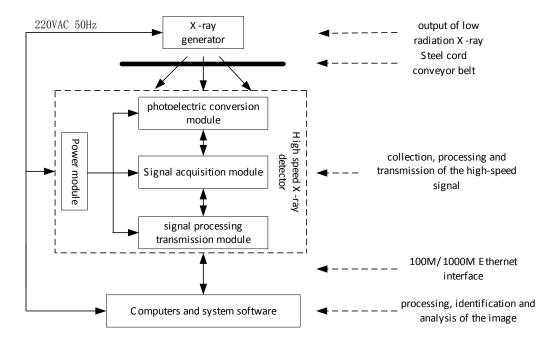
Fig. (1). The structure frame of steel cord conveyor belt detection system.
