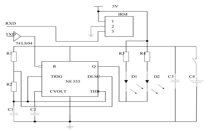
Fig. (4). Infrared transmitting and receiving circuit.
