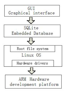
Fig. (3). The master control platform architecture of ARM noise data control module.
