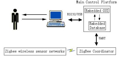
Fig. (2). The working schematic diagram of noise data control module.
