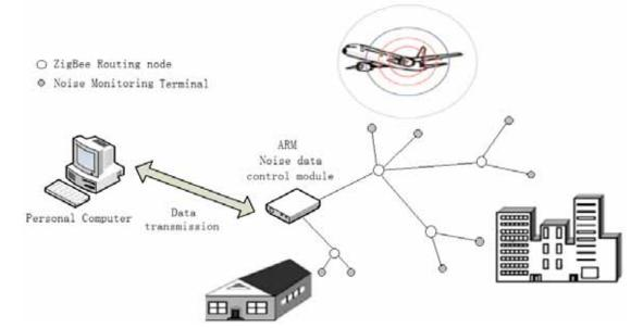
Fig. (1). The airport noise data collection system based on wireless sensor networks.
