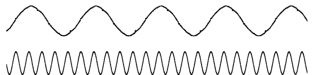
Zero-sequence voltage wave of point a and zero-sequence voltage fifth harmonic component wave of point b
