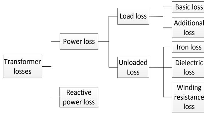
Fig. (2). Composition transformer losses.
