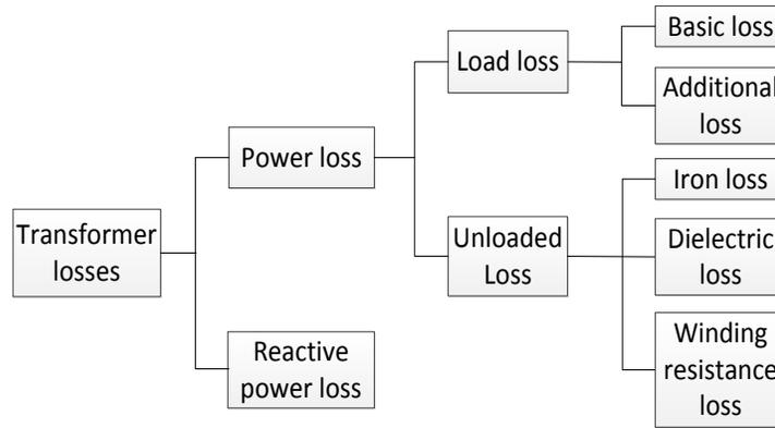
Fig. (2). Composition transformer losses.
