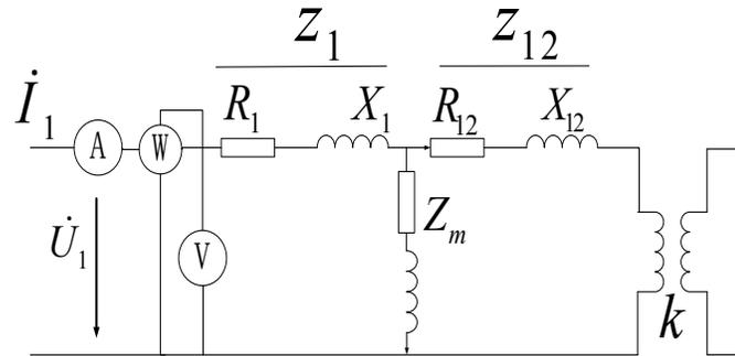
Fig. (1). Wiring diagram of short circuit test method.
