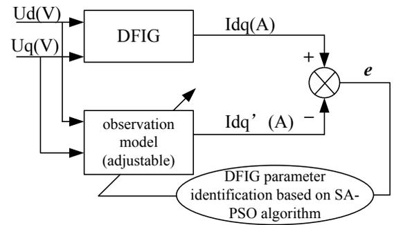
Fig. (2). Diagram of the Parameter Identification Based on SA-PSO Algorithm.
