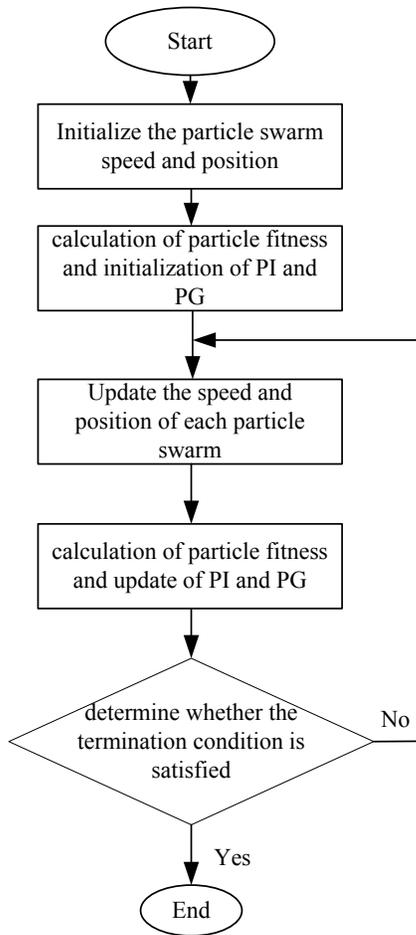
Fig. (1). Flow Chart of PSO Algorithm.
