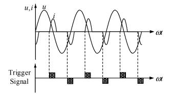
Fig. (2). Waveform of Power System Voltage and TCR Current.
