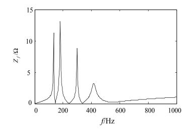
Fig. (12). Impedance-frequency Characteristics of PPF.
