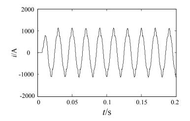
Fig. (4). Waveform of the Current Which TCR Injecting Into Phase c under Symmetrical Voltage.
