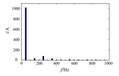
Fig. (7). Frequency Spectrum of the Current Which TCR Injecting into Phase C under Asymmetrical Voltage.
