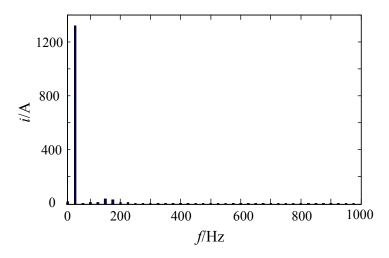
Fig. (11). Current Frequency Spectrum of Power System after PPF Operating.
