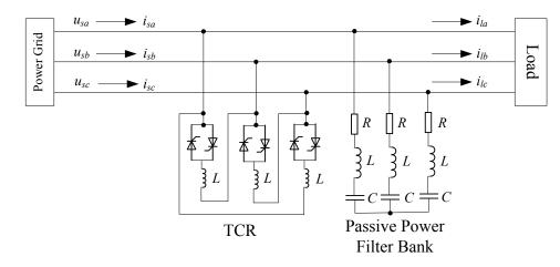
Fig. (1). Topology of TCR Compensation System.
