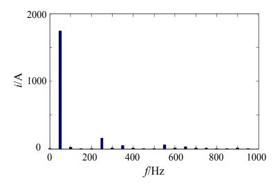
Fig. (9). Current Frequency Spectrum of Power System before PPF Operating.
