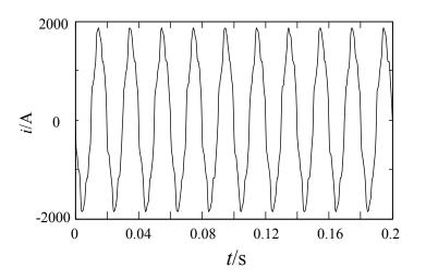
Fig. (8). Current Waveform of Power System before PPF Operating.
