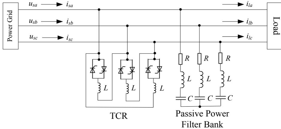
Fig. (1). Topology of TCR compensation system.
