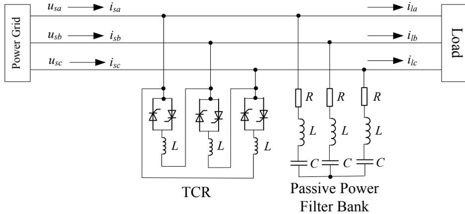
Fig. (1). Topology of TCR compensation system.
