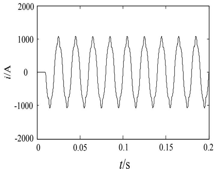
Fig. (6). Waveform of current which TCR injecting into phase C under asymmetrical voltage.
