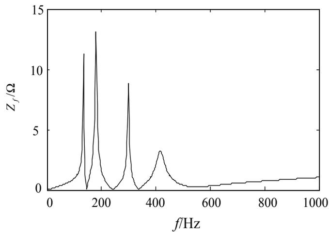
Fig. (12). Impedance-frequency characteristics of PPF.
