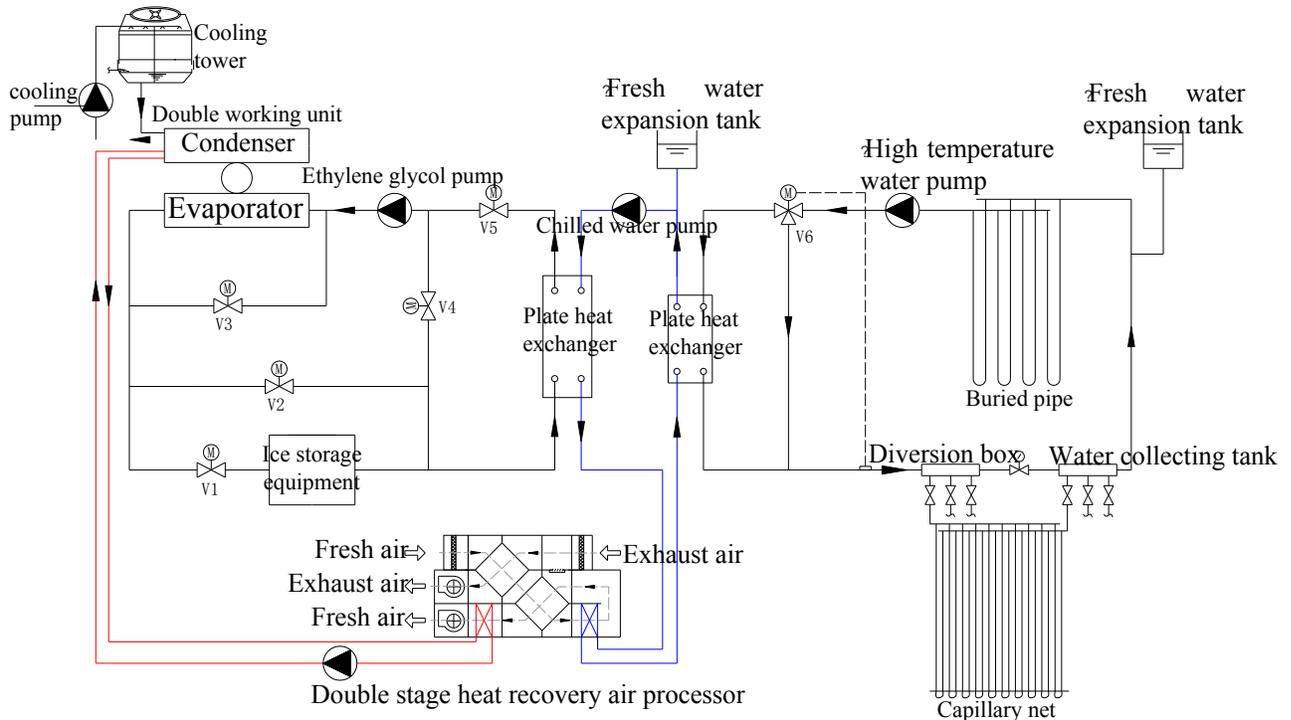
Fig. (1). Schematic diagram of air-conditioning system.
