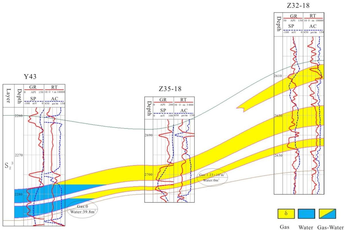
Fig. (7). Connecting-well profile of gas and water for the Y43—Z35-18—Z32-18 wells.
