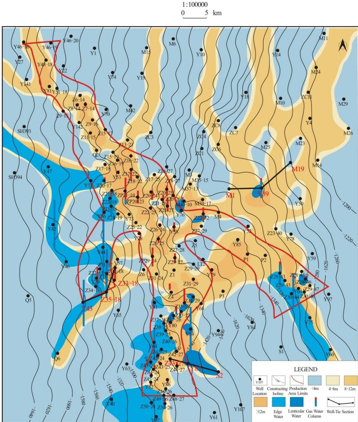
**Fig. (9).** Superimposed plan of water bodies and sand bodies and the superstructure of the Shan 2<sup>3</sup> member in the Zizhou gas field.
