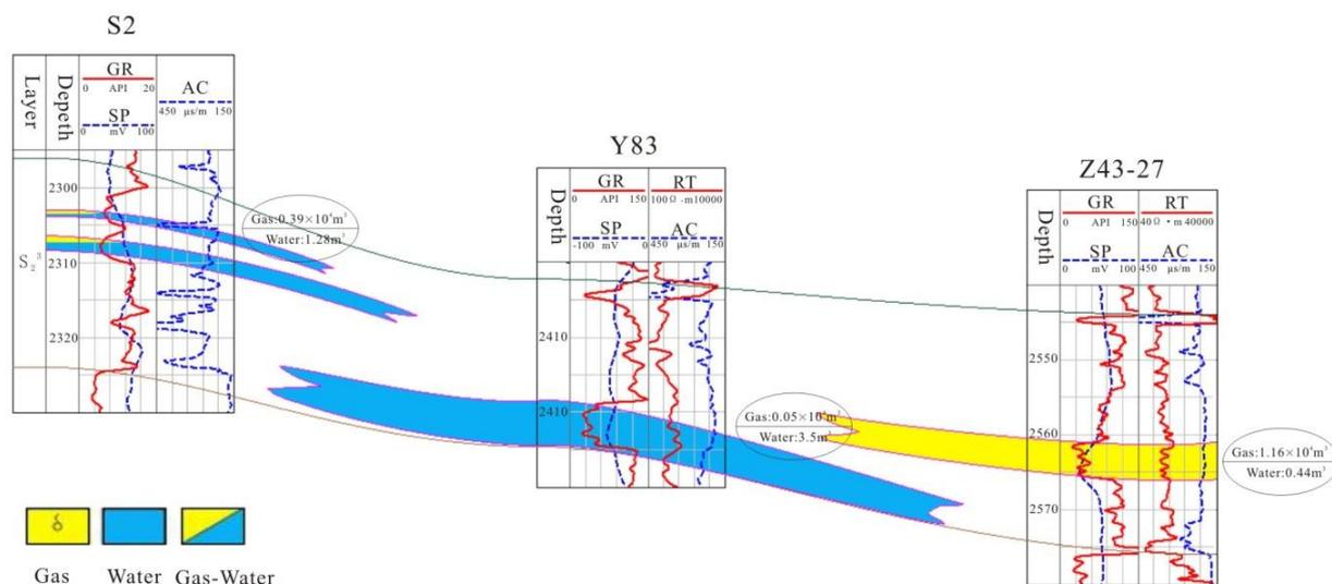
Fig. (8). Connecting-well profile of gas and water for the S2—Y83—Z43-27 wells.
