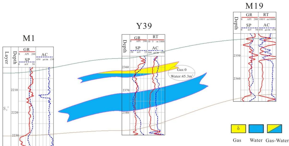
Fig. (5). Typical profile of the lenticular water.
