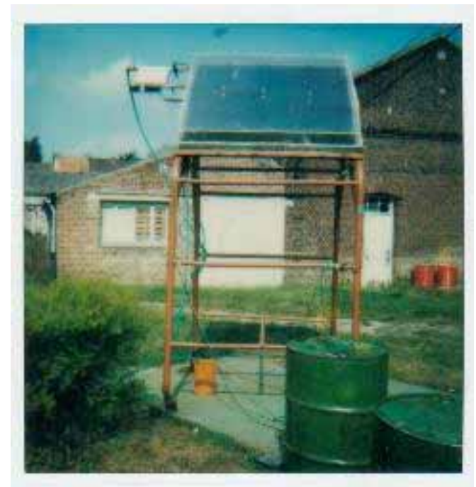
Fig. (4). Pump housing with the cooling reserve.
