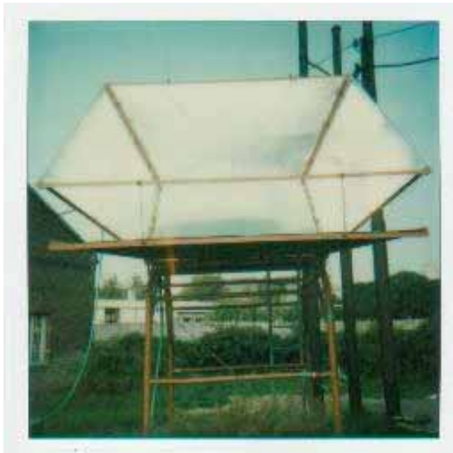
Fig. (5). the pump with its reflectors.
