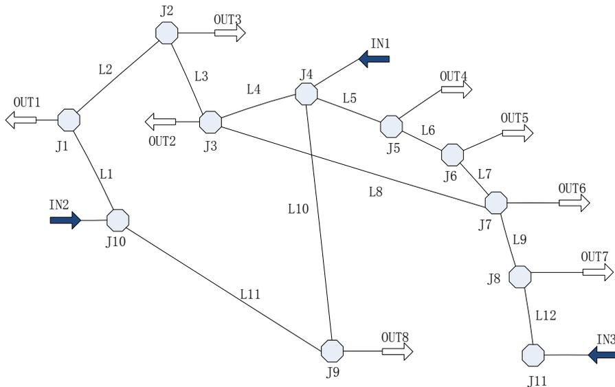
Fig. (2). Structure of pipeline network.
