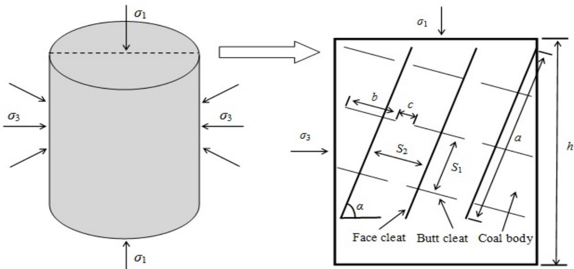
Fig. (1). Mechanical model of cleats combined coal body.
