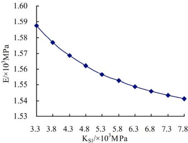
Fig. (5). The relationship between the elastic modulus  $E$  of coal body and the shear stiffness  $k_{s1}$  of butt cleat.
