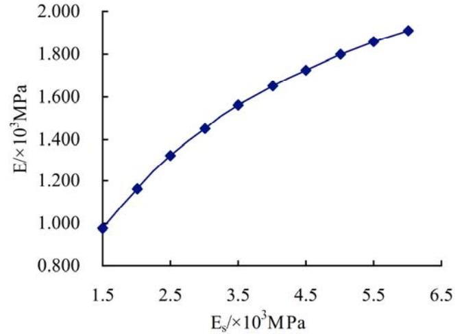
**Fig. (2).** The relationship between the elastic modulus  $E$  of coal body and the elastic modulus  $E_s$  of coal rock block.
