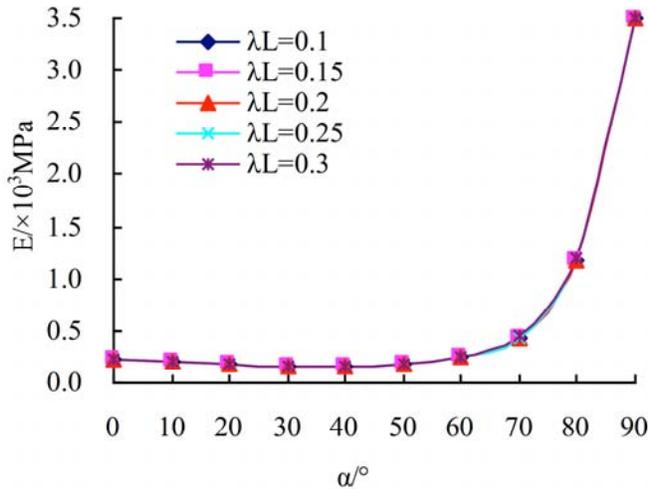
Fig. (9). The relationship among the elastic modulus  $E$  of coal body, inclination  $\alpha$  of face cleat and the connectivity rate  $\lambda_L$  of butt cleats.
