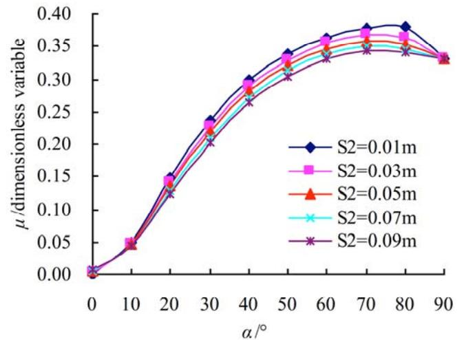
Fig. (11). The relationship among the Poisson's ratio  $\mu$  of coal body, inclination  $\alpha$  of face cleat and the distance  $S_2$  between face cleats.
