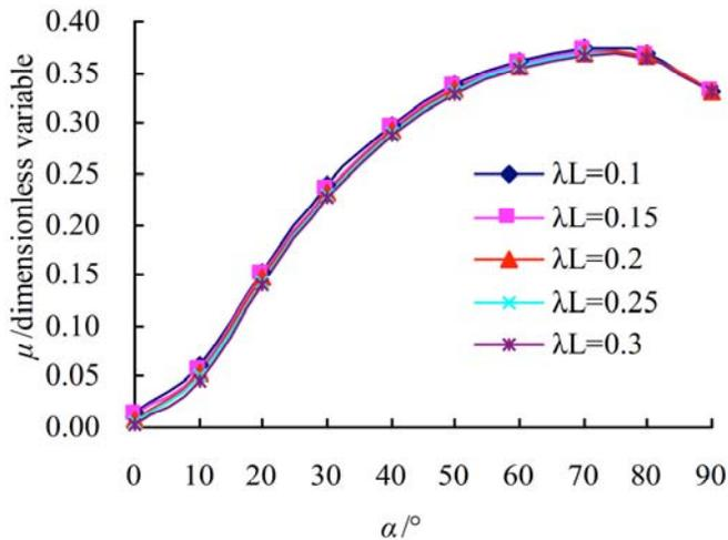
**Fig. (12).** The relationship among the Poisson's ratio  $\mu$  of coal body, inclination  $\alpha$  of face cleat and the connectivity rate  $\lambda_L$  of butt cleats.
