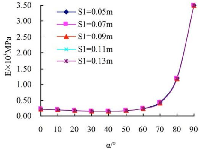
Fig. (7). The relationship among the elastic modulus  $E$  of coal body, inclination  $\alpha$  of face cleat and the distance  $S_1$  between butt cleats.
