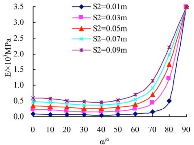
Fig. (8). The relationship among the elastic modulus  $E$  of coal body, inclination  $\alpha$  of face cleat and the distance  $S_2$  between face cleats.
