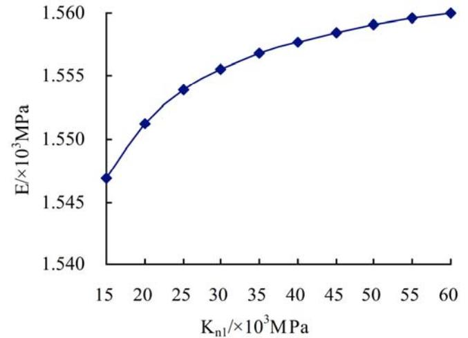
**Fig. (3).** The relationship between the elastic modulus  $E$  of coal body and the normal stiffness  $k_{n1}$  of butt cleat.
