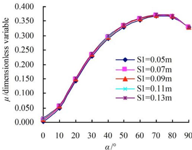
Fig. (10). The relationship among the Poisson's ratio  $\mu$  of coal body, inclination  $\alpha$  of face cleat and the distance  $S_1$  between butt cleats.
