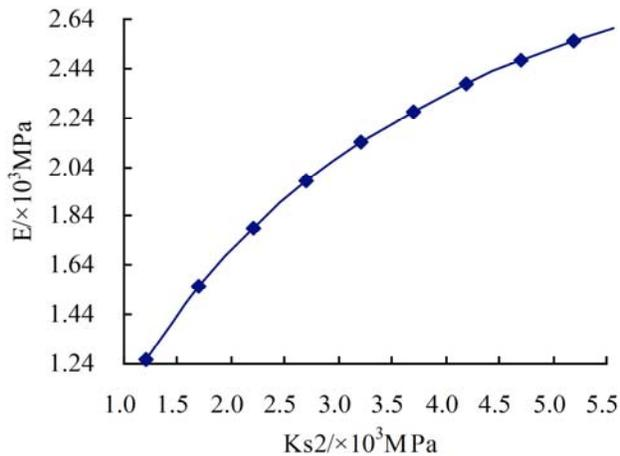
Fig. (6). The relationship between the elastic modulus  $E$  of coal body and the shear stiffness  $k_{s2}$  of face cleat.
