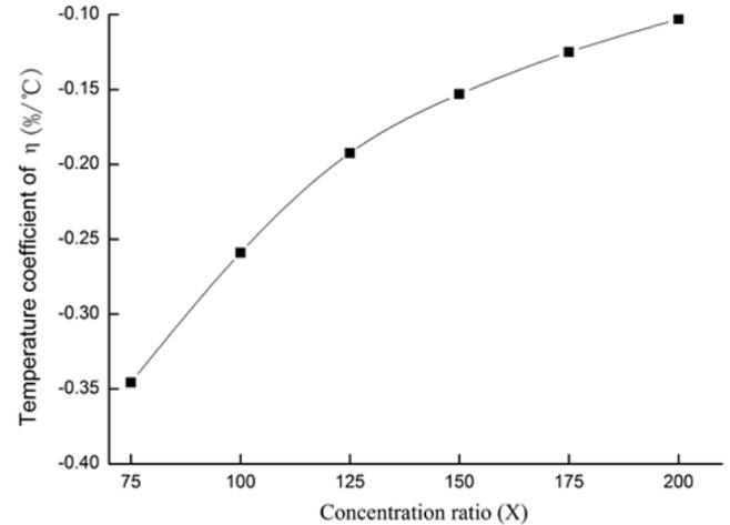
Fig. (9). The temperature coefficient of  $\eta_c$  as a function of concentration ratio.
