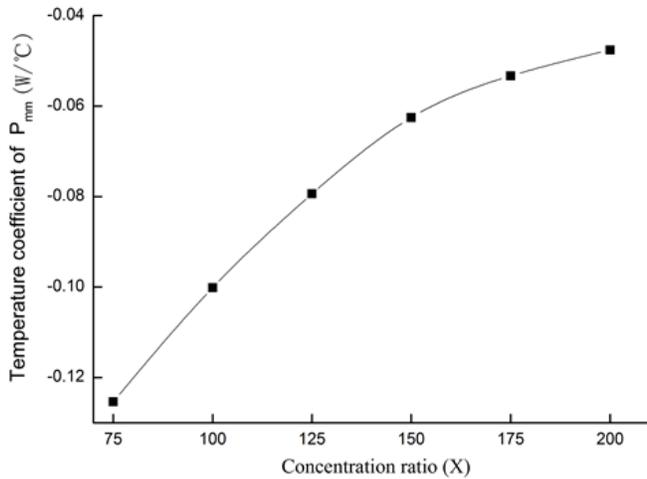
Fig. (7). The temperature coefficient of  $P_{mm}$  as a function of concentration ratio.
