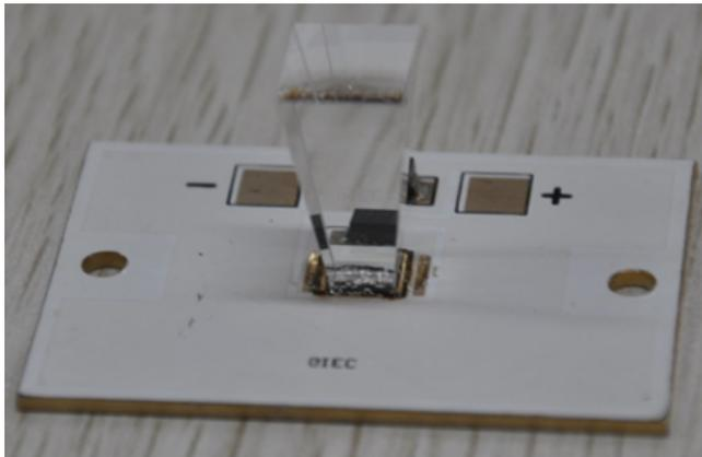
Fig. (4). The three junction GaInP/GaInAs/Ge solar cell with homogenizer.
