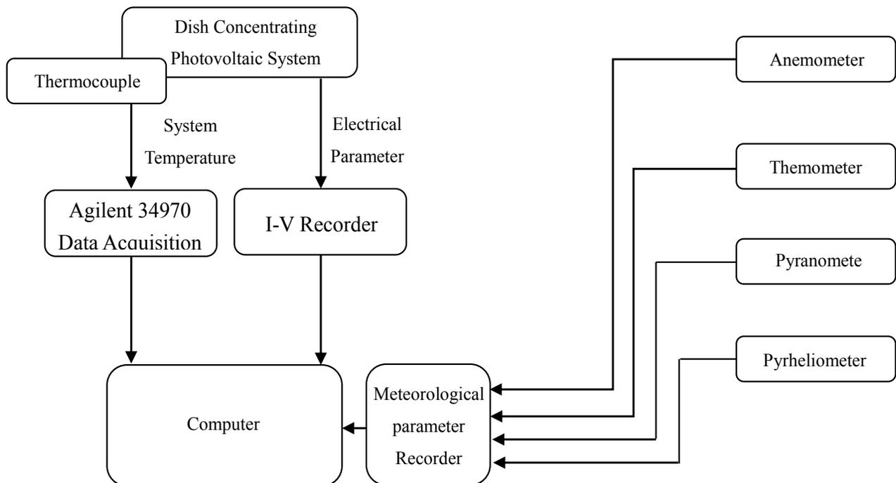
Fig. (3). Dish concentrating photovoltaic system performance test platform.
