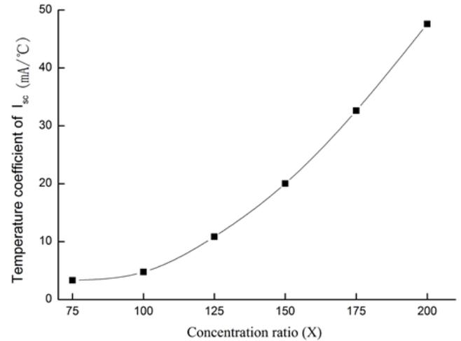
Fig. (6). The temperature coefficient of  $I_{sc}$  as a function of concentration ratio.
