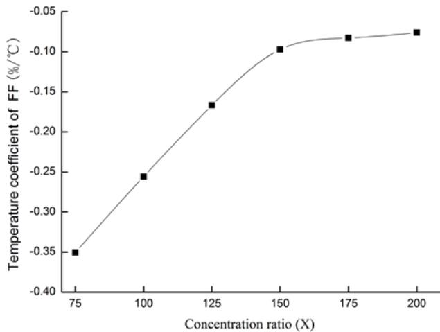
Fig. (8). The temperature coefficient of  $FF$  as a function of concentration ratio.
