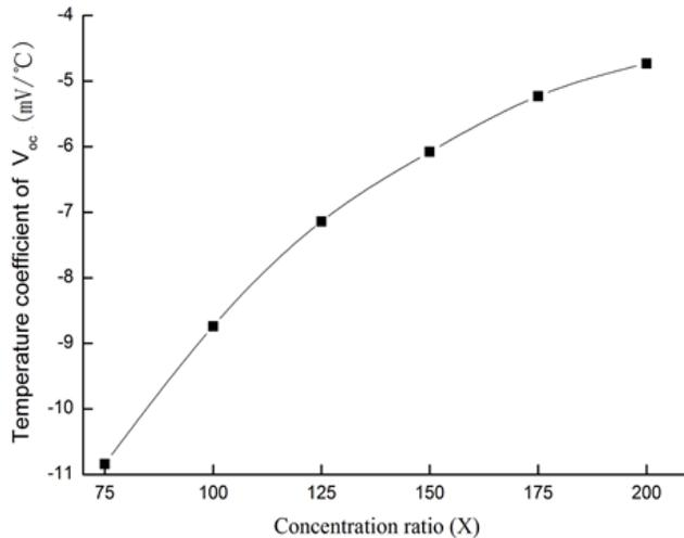
Fig. (5). The temperature coefficient of  $V_{oc}$  as a function of concentration ratio.
