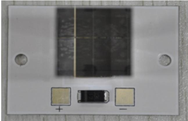
Fig. (2). Three junction GaInP/GaInAs/Ge solar cell.
