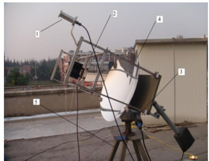
1-solar monitor; 2-solar cell module; 3-transmission mechanism; 4- concentrator; 5- Support
