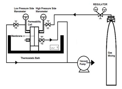
Fig. (1). Schematic view of the equipment used in the separation test.
