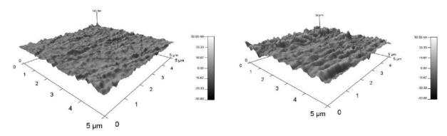
Fig. (4). AFM plot of 5 wt % and 10 wt % membranes (scale of 5  $\mu$ m  $\times$  5  $\mu$ m).
