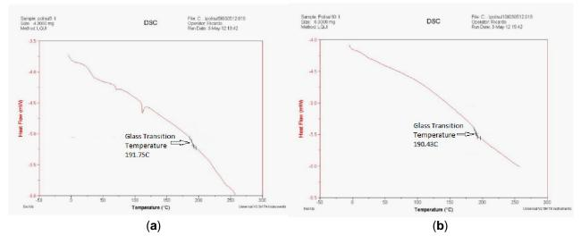
Fig. (2). DSC curves for (a) 5% wt and (b) 10% wt membranes.
