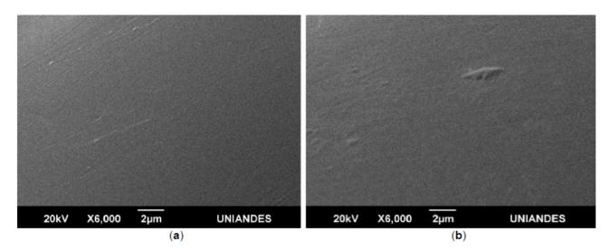
Fig. (3). SEM images of a) 5% wt and b) 10% wt membranes.
