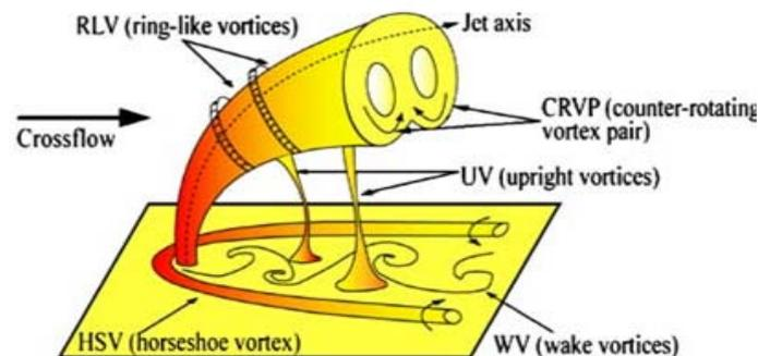
Fig. (1). Vortex structure of a JICF [13].
