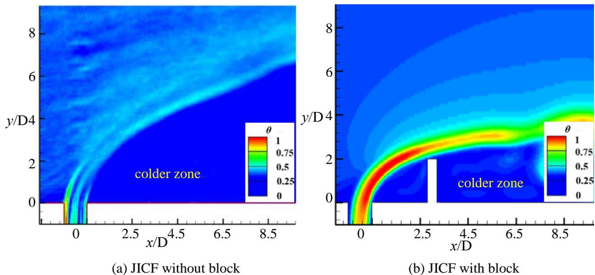
Fig. (6). Temperature field on the iso-surface at  $r=3$ .
