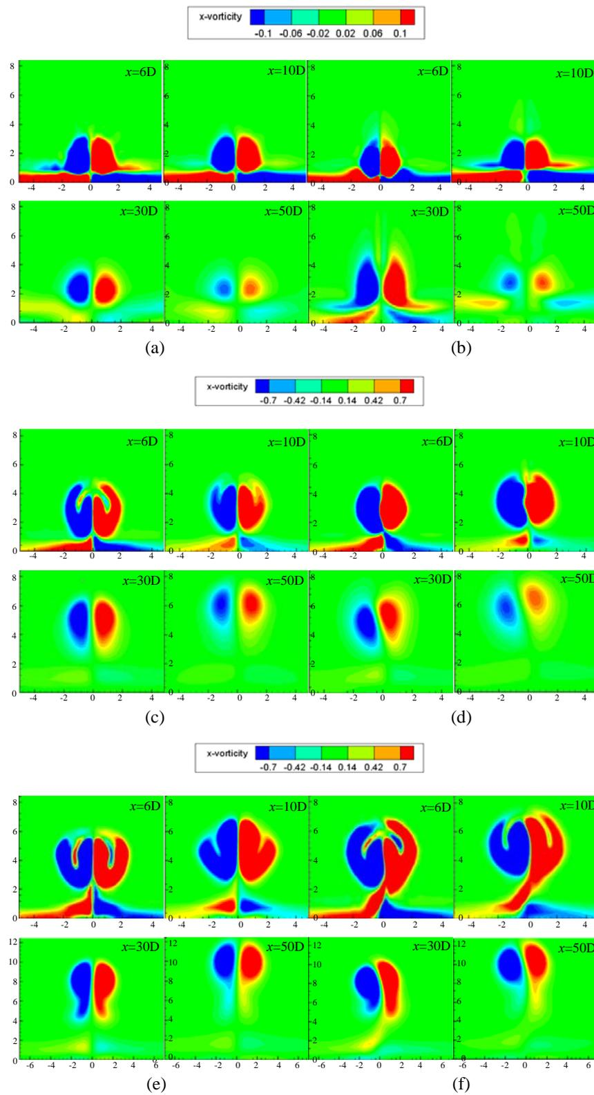
**Fig. (5).** Spanwise vorticity at different distance ((a). JICF without block at  $r=1$ ; (b). JICF with block at  $r=1$ ; (c). JICF without block at  $r=2$ ; (d). JICF with block at  $r=2$ ; (e). JICF without block at  $r=3$ ; (f). JICF with block at  $r=3$ )
