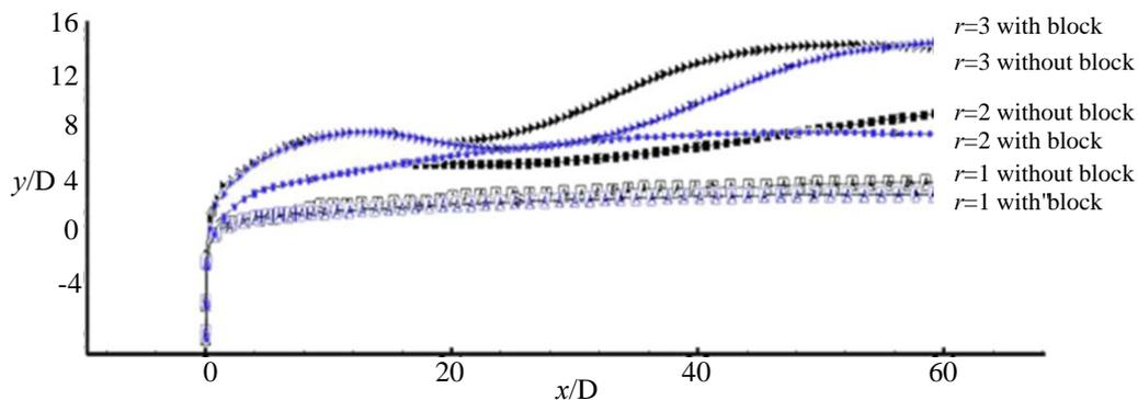
Fig. (3). Time-averaged particle trajectories for the JICF (Black: cases without block; blue: cases with block).
