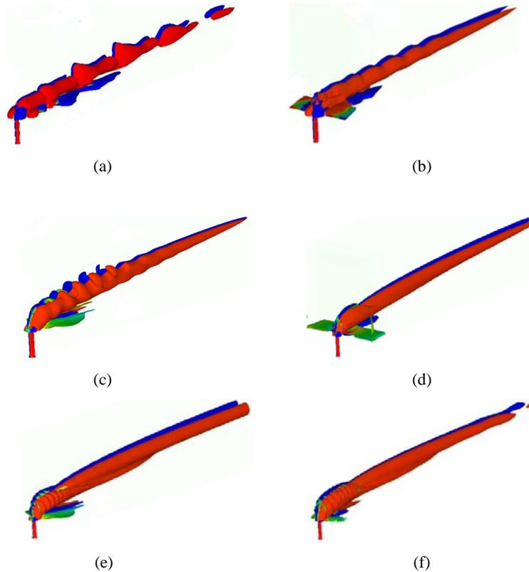
**Fig. (4).** Three dimensional vortex structures for the JICF with and without block ((a). JICF without block at  $r=1$ ; (b). JICF with block at  $r=1$ ; (c). JICF without block at  $r=2$ ; (d). JICF with block at  $r=2$ ; (e). JICF without block at  $r=3$ ; (f). JICF with block at  $r=3$ )
