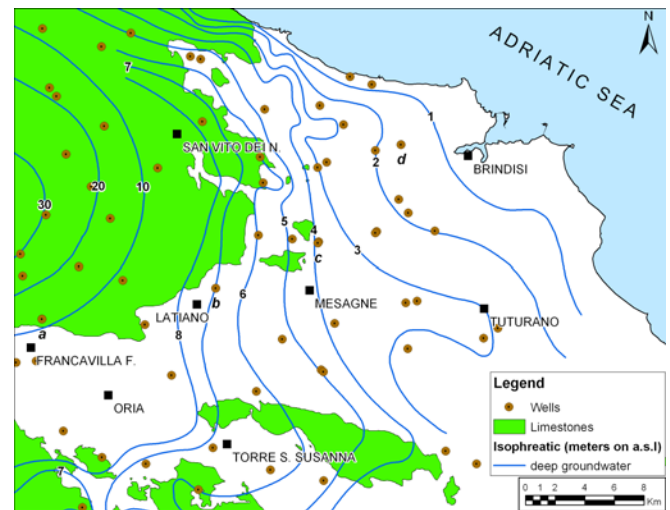
Fig. (6). Piezometric surface of deep groundwater; letters mark the wells used for chemical characterization of deep groundwater (see figure 7).
