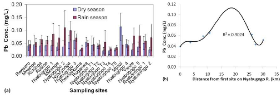
Fig. (17). Lead levels for (a) all the sampling sites and (b) sampling sites located on the Nyabugogo River for the monitored period.
