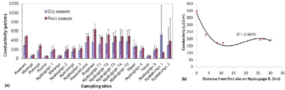
Fig. (4). Conductivity levels for (a) all the sampling sites and (b) sampling sites located on the Nyabugogo River for the monitored period.
