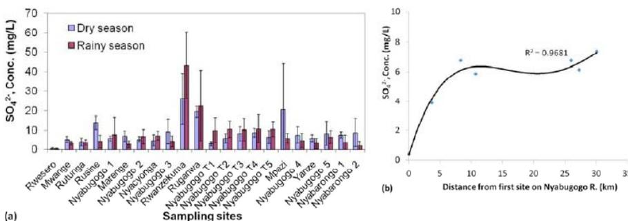
Fig. (11). Sulphate levels for (a) all the sampling sites and (b) sampling sites located on the Nyabugogo River for the monitored period.
