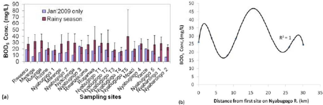
Fig. (13). BOD<sub>5</sub> levels for (a) all the sampling sites and (b) sampling sites located on the Nyabugogo River for the monitored period.
