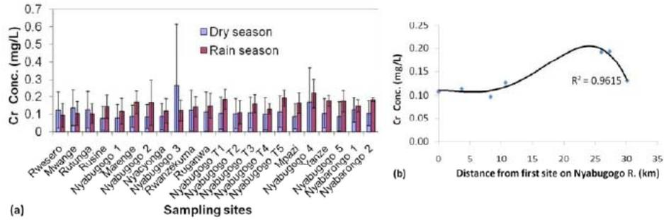
Fig. (18). Chromium levels for (a) all the sampling sites and (b) sampling sites located on the Nyabugogo River for the monitored period.
