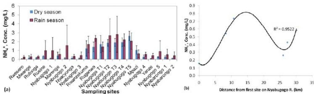
Fig. (8). NH<sub>4</sub>-N levels for (a) all the sampling sites and (b) sampling sites located on the Nyabugogo River for the monitored period.
