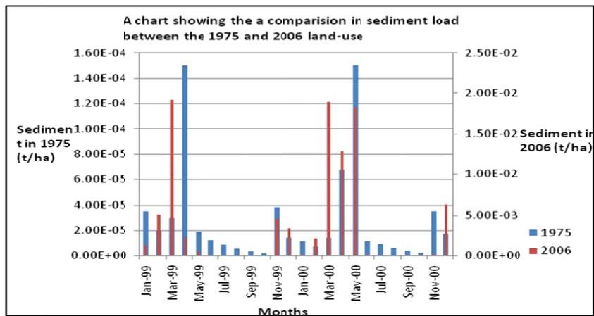
Fig. (2). Comparative analysis of sediment yields based on land uses in the Simiyu Catchment for 1975 and 2006(Source: [9, 10]).
