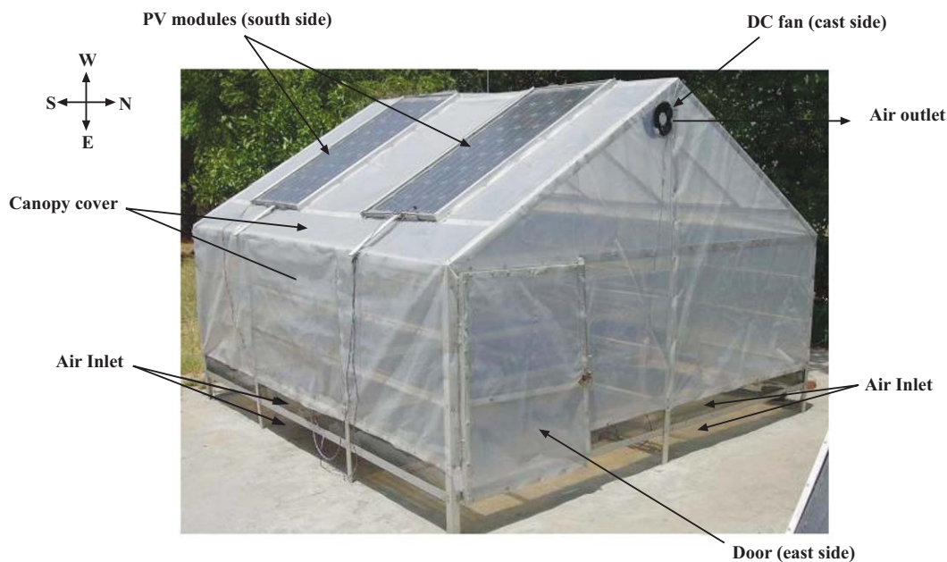
Fig. (1). Photograph of hybrid photovoltaic/thermal greenhouse dryer [6,7].
