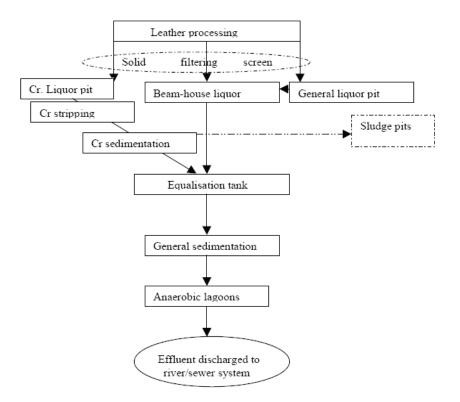
Fig. (1). Flow diagram illustrating effluent treatment in a typical leather processing site in Kenya [11].
