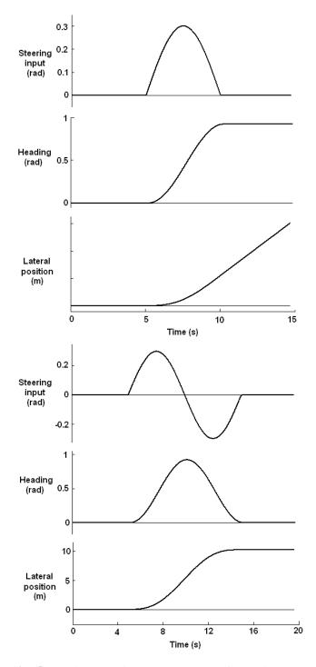
**Fig. (5).** Steering wheel inputs necessary to perform a simple turn (top) and a lane change (bottom).
