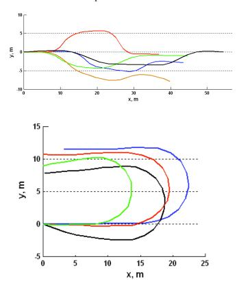
**Fig. (4).** Typical tractor trajectories as the tractor operator performed maneuvers 1 and 5 in the field.
