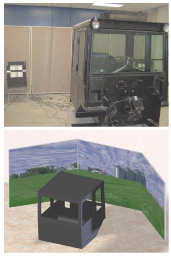
**Fig. (2).** The front view of the simulator (top) and a schematic representation of the simulator and the visual display during operation (bottom).
