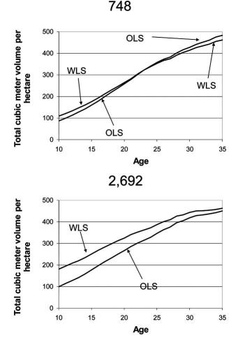
**Fig. (2).** Predicted total cubic meter outside-bark volume per hectare for two planting densities (748 and 2,692) as estimated using PTAEDA 3.1. Parameters of the combined-variable volume equation were estimated using weighted least squares (WLS) and ordinary least squares (OLS). Volumes were predicted in cubic feet per acre and then converted to cubic meters per hectare using a multiplier of 0.06997.
