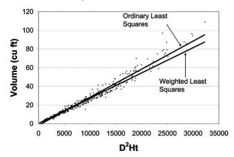
Fig. (1). Plot of all 431 individual tree total cubic foot outside-bark volume observations plotted over  $D^2Ht$  (D = in. and Ht = ft). Predictions of total cubic foot volume when using ordinary least squares [equation 4] and weighted least squares [equation 5] are also presented.
