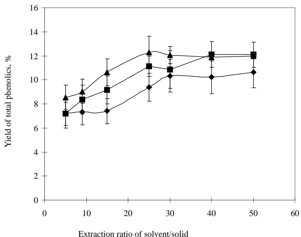
**Fig. (5).** The effect of the ratio of solvent /solid ( $\text{gg}^{-1}$ ) used in the extraction on the yield of total phenolics. The extraction time was 2 min and the particle size of 40 mesh was used. ◆, 25°C; ■, 60°C; ▲, 95°C.
