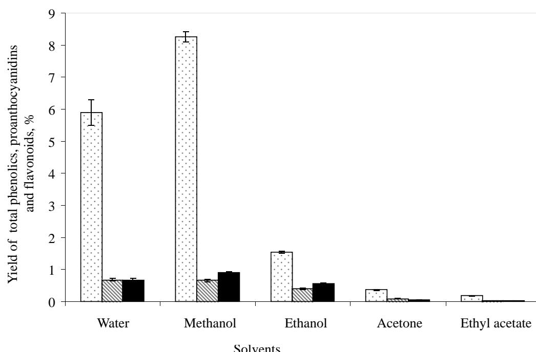
**Fig. (1).** The effect of different solvents on the yield of total phenolics, proanthocyanidins and flavonoids from the marc of pomegranate peels. Extraction was conducted at a temperature of  $40^\circ\text{C}$ , a solvent/solid ratio of 15:1, a particle size of 40 mesh and an extraction time of 240 min: □, Total phenolics; ▨, Proanthocyanidins; ■, Flavonoids.
