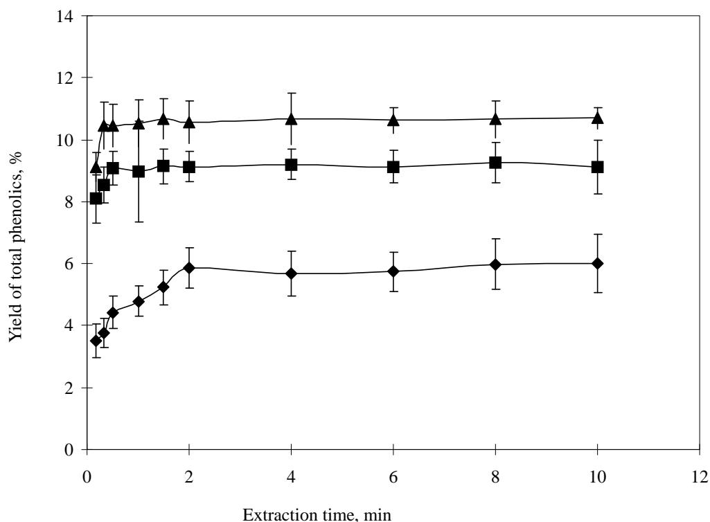
**Fig. (3).** The kinetics curves of water extracted total phenolics yield. The water extraction was done using a ratio of solvent to solid of 15: 1 and particle size of 40 mesh. —◆—, 25°C; —■—, 60°C; —▲—, 95°C.
