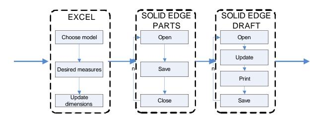
Fig. (6). General implementation architecture for flexible design of lockers.
