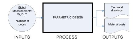
Fig. (5). Implementation process for parametric designs.
