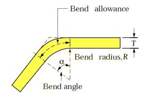
Fig. (3). Neutral axis in bending operations.
