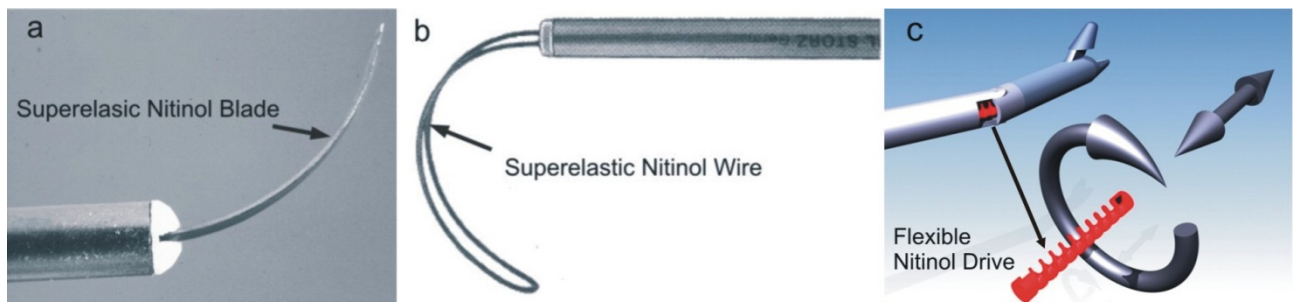
Fig. (2). Variable-curvature devices for laparoscopic surgery. a) Dissecting spatula, b) suture passer, c) flexible drive for an articulating needle holder. (From [29], reproduced with permission from Springer).
