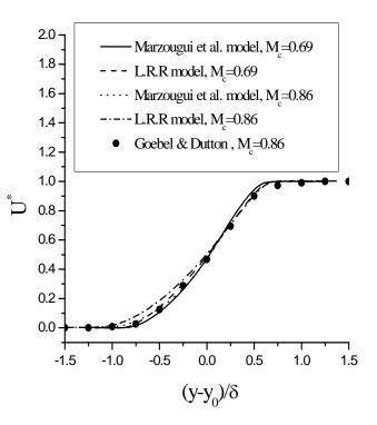
Fig. (1). Similarity profiles of mean stream wise velocity.
