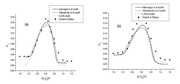
Fig. (2). Similarity profile of longitudinal turbulence intensity: (a)  $M_c = 0.69$ , (b)  $M_c = 0.86$ .
