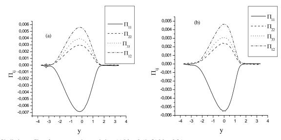
Fig. (5). Similarity profiles of pressure-strain correlation: (a)  $M_c = 0.69$ , (b)  $M_c = 0.86$ .
