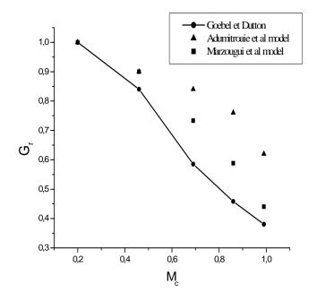
**Fig. (6).** Normalized growth rate G<sub>r</sub> versus convective Mach number.
