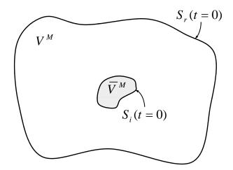
**Fig.** (1). Geometry of the hydride precipitation problem in the reference configuration (t=0). The shaded area of the metal, of volume  $\bar{V}^M$  ( $\bar{V}^M << V^M$ ), transforms into a hydride. When the transformation occurs under stress, as in Section 4, traction is applied on the external boundary.
