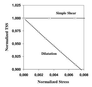
Fig. (2). Effects of applied stress on normalized hydrogen terminal solid solubility,  $C^{TS}/C_{\ell}^{TS}$ , of Zircaloy-2 at 573 K, in the case of dilatation and simple shear, where the normalized stress is given by  $S_D/K$  and  $S_S/\mu$ , respectively.
