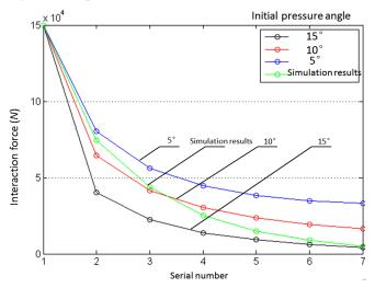
Fig. (15). Comparison of chain links tension.
