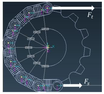
Fig. (13). Assembly model of meshing area.
