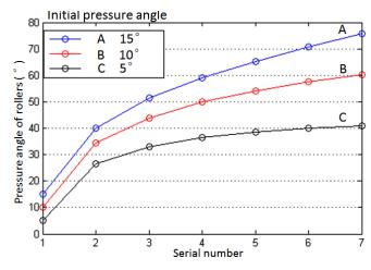
Fig. (7). The effect of initial pressure angle.
