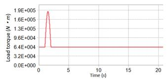
Fig. (18). Load torque on driving sprocket.
