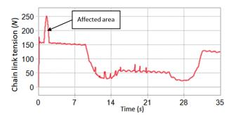
Fig. (20). Tension in tight-side chain.
