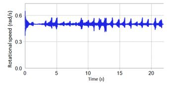
Fig. (19). Rotation speed of the driven sprocket.
