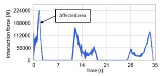
Fig. (22). Forces between roller and driving sprocket.
