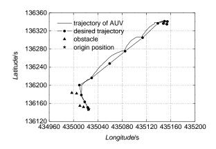
Fig. (15). Voyage trace of "ZT-AUV".
