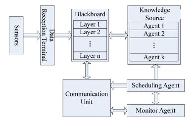
Fig. (4). Structure of blackboard system.
