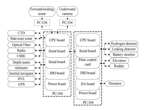
Fig. (9). Structure of embedded motion control system.
