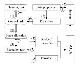
Fig. (10). Data flow of embedded motion control system.
