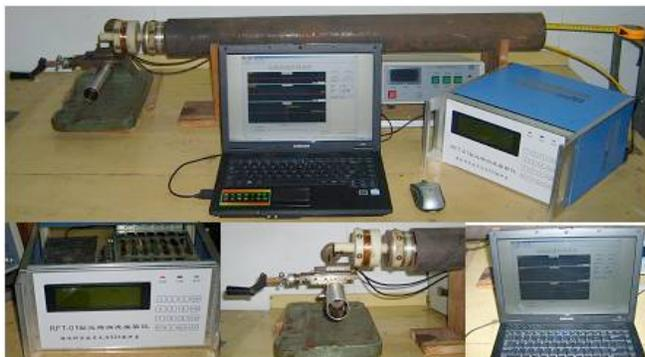
Fig. (8). Principle and photography of detection system.
