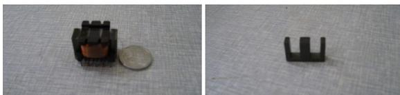
Fig. (11). Differential radial field detection coil.
