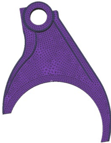
Fig. (2). Grid meshing result of shift fork.
