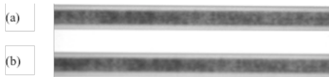
Fig. (3). Image pre-processing of Nonel tube: (a) Image affected by noise; (b) Image processed by mean filter.
