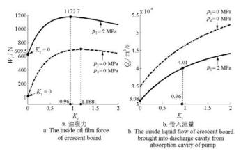
Note: sign  $W_i$  indicates the inside oil film force of crescent board, N; sign  $Q_i$  indicates the inside liquid flow of crescent board brought into discharge cavity from absorption cavity of pump,  $m^3/s$ ; sign  $K_i$  indicates the convergence ratio of inside radial convergent gap of crescent board, similarly hereinafter.
