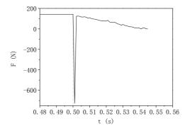
Fig.8 The curve of valve spool by fluid pressure in shuttle check valve during closing processat
