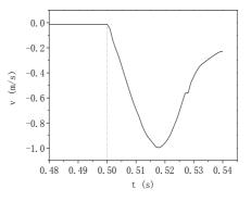
Fig.10 The curve of velocity vectors of valve spool in shuttle check valve during closing process
