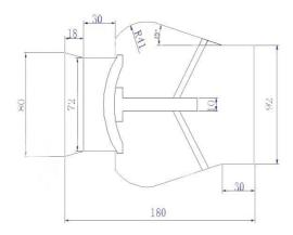
Fig.2 model diagram of shuttle valve
