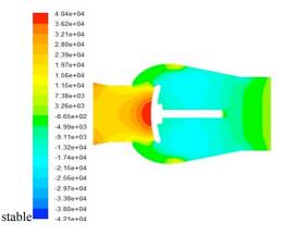
Fig.5 Pressure contour in shuttle check valve in the
