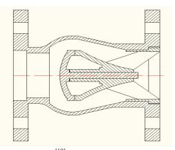
backpressure <sup>[10]</sup>. Functionally speaking, the shuttle check valve can function as opening and closing, throttling, damping, and amplify regulator and controller.
