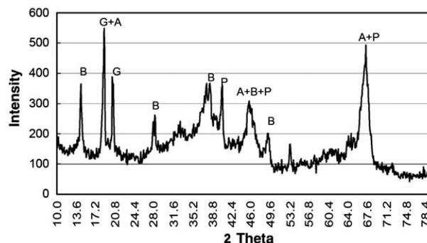
**Fig. (1).** The XRD pattern of the spent catalyst sample before leaching [11]. B = boehmite (syn.-  $\text{AlOOH}$ ), A =  $\gamma\text{-Al}_2\text{O}_3$ , G = gibbsite  $\text{Al}(\text{OH})_3$ , P = palladium.
