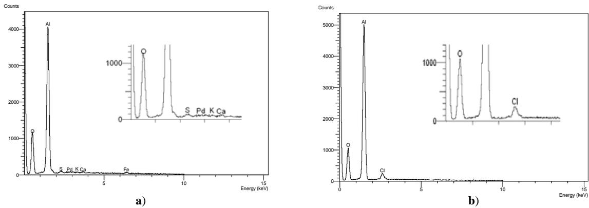
**Fig. (2) The XRD pattern of the spent catalyst sample. a) Before leaching (oxygen, aluminum, sulfur, potassium, calcium, and palladium). b) After leaching (oxygen, aluminum, and chlorine).**
