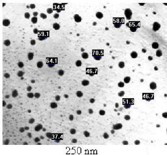
**Fig. (8).** The TEM pattern for electroless deposited Pd from waste solution. 60 KV and 40000 magnification power.
