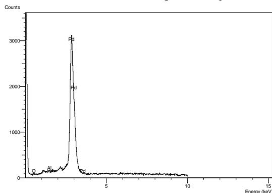
**Fig. (9).** EDX analysis for electroless deposited Pd from waste solution.
