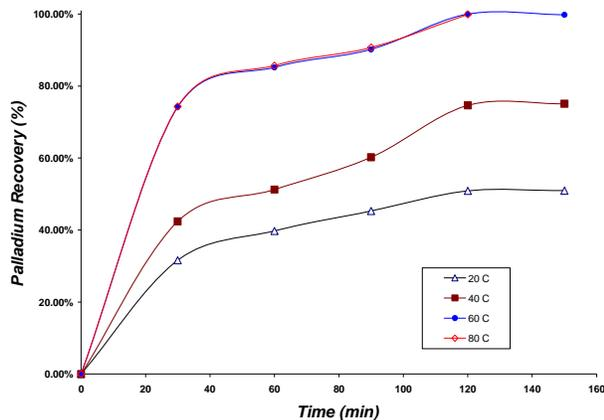
**Fig. (4). The recovery of Pd as a function of time and temperature. With 10% HCl, 5% AlCl<sub>3</sub> and L/S = 20.**
