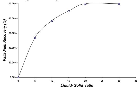
**Fig. (6)** The effect of liquid/ solid ratio (L/S) on Pd recovery. With 10% HCl and 5% AlCl<sub>3</sub> at 60 °C for 2 hours.
