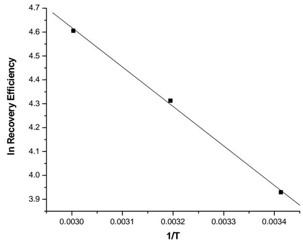
**Fig. (5). The Arrhenius plot for the leaching process. 10% HCl, 5% AlCl<sub>3</sub>, 2 hours and L/S = 20.**
