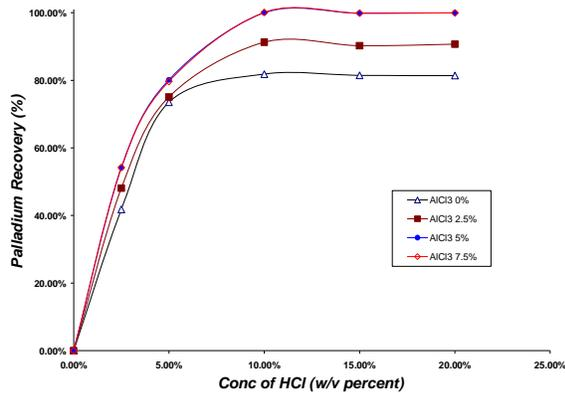
**Fig. (3). The effect of the hydrochloric acid concentration on the efficiency of Pd recovery. With different concentration of AlCl<sub>3</sub> measured after 2 hours at 80 °C, with ratio L/S = 20.**
