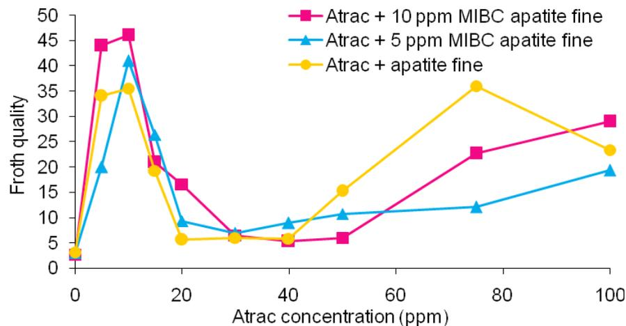
Fig. (18). Froth quality in the presence of fine apatite particles and with and without frother as a function of collector concentration.
