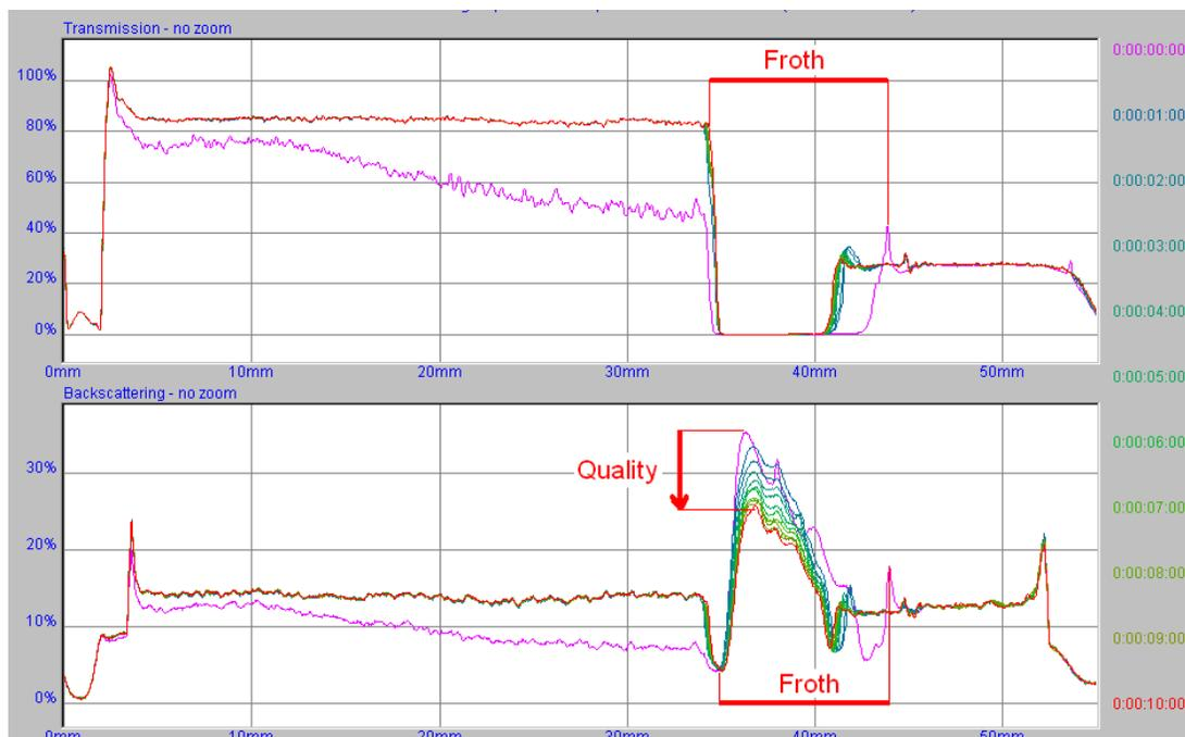
**Fig. (1).** Turbiscan measurement and data outcome used for the analysis.
