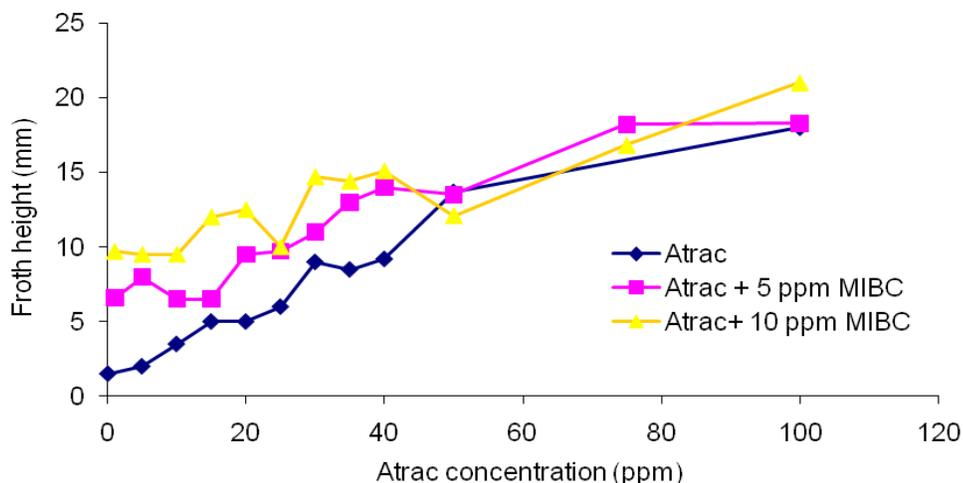
Fig. (10). Froth formation in the absence and presence of frother as a function of collector concentration at pH 8.5.
