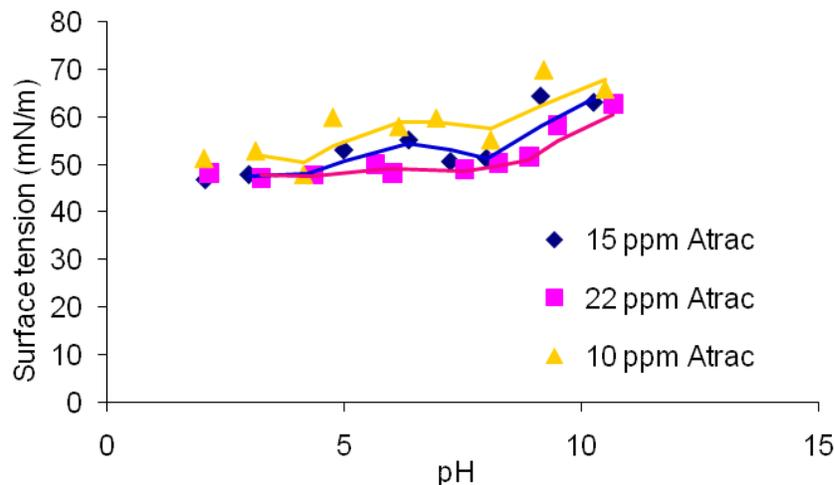
**Fig. (4).** Surface tension of aqueous solutions of collector as a function of pH at three initial concentrations.
