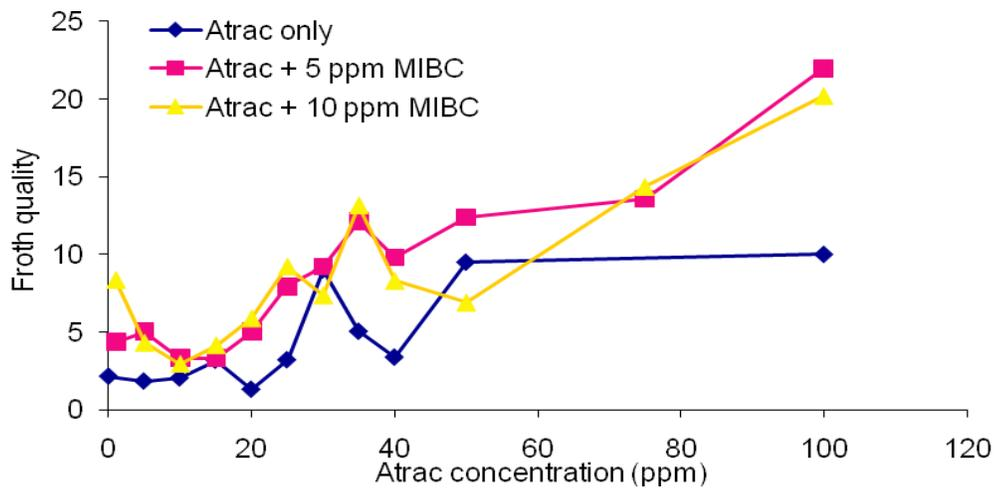
**Fig. (11).** Froth quality in the absence and presence of frother as a function of collector concentration at pH 8.5.
