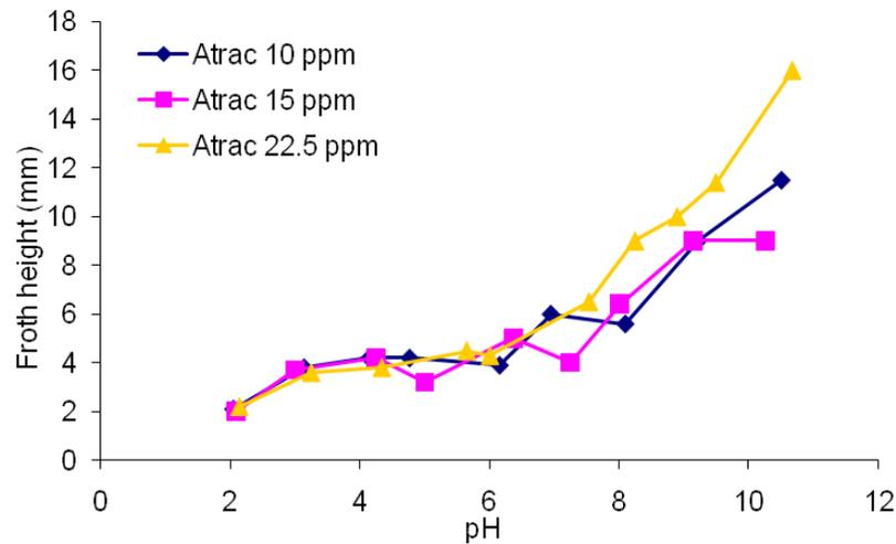
Fig. (9). Influence of pH on froth formation of different concentrations of collector solutions.
