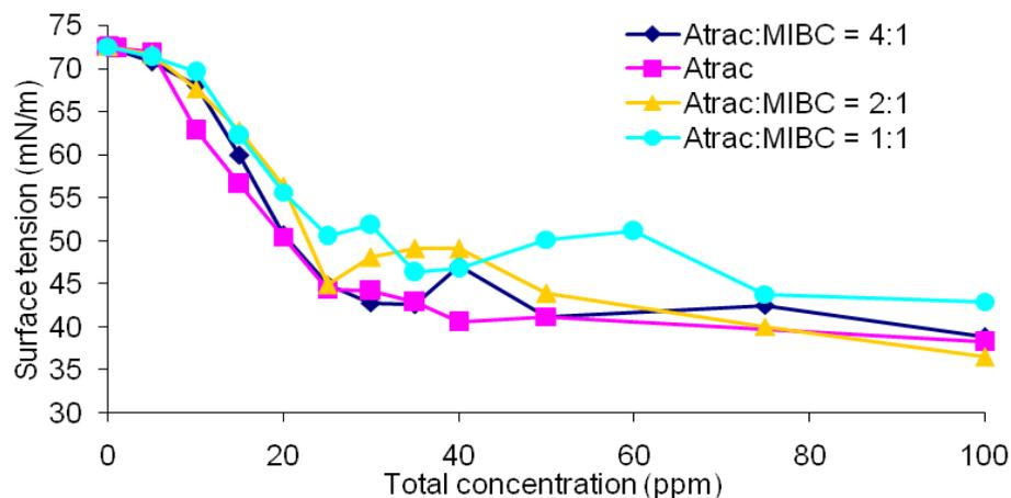
Fig. (7). Surface tension of aqueous solutions of collector and frother at different compositions as a function of total concentration at pH 8.5.
