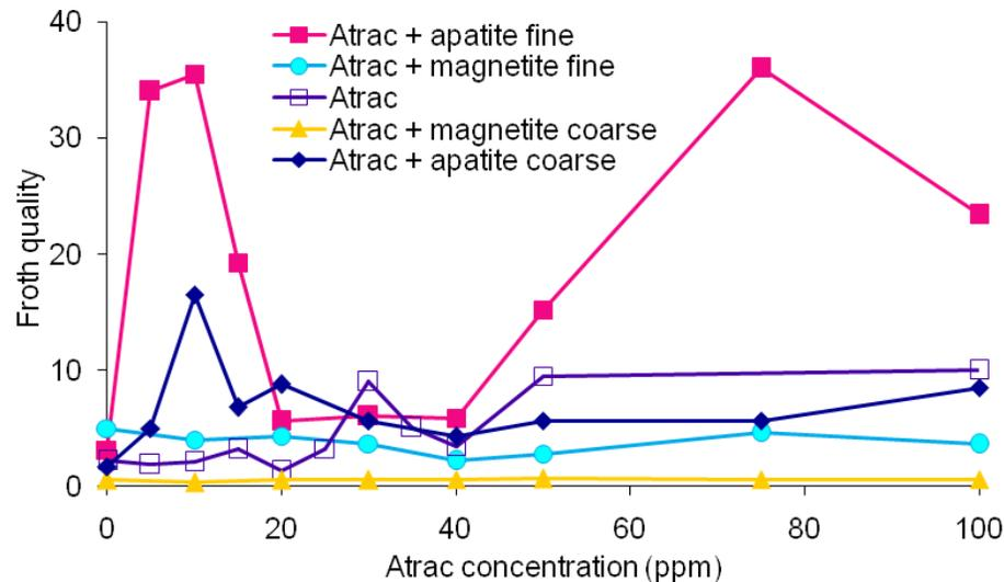
**Fig. (15).** Froth quality in the presence of apatite and magnetite particles as a function of collector concentration.
