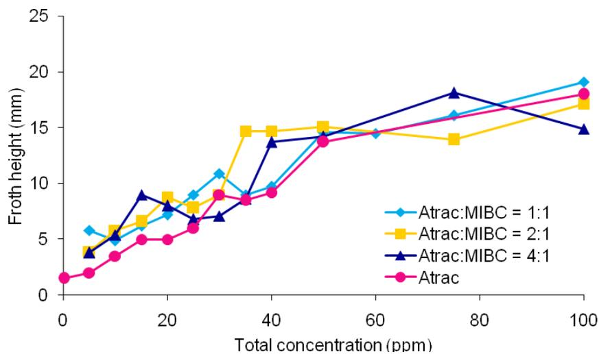
**Fig. (12).** Froth formation at different collector and frother composition as a function of total concentration at pH 8.5.
