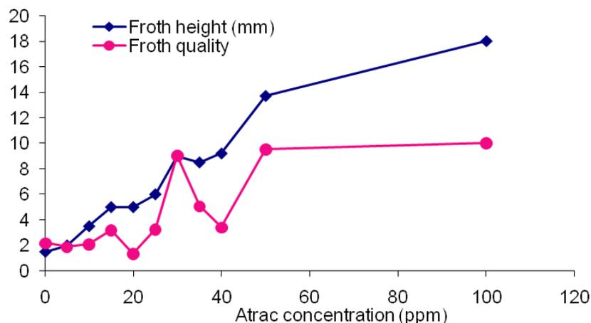
Fig. (8). Froth height and quality as a function of collector concentration at pH 8.5.
