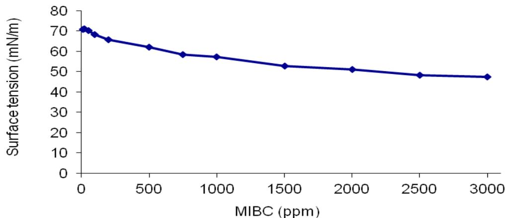
**Fig. (3).** Surface tension of aqueous solution of MIBC frother at pH 8.5.
