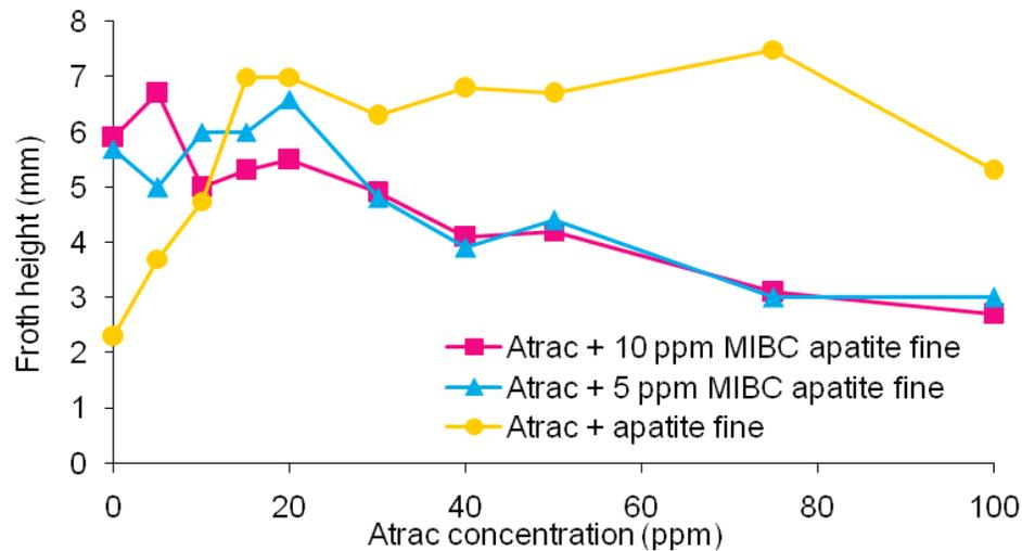
Fig. (17). Froth formation in the presence of fine apatite particles and with and without frother as a function of collector concentration.
