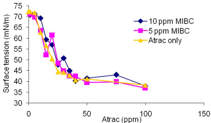
Fig. (6). Surface tension of collector aqueous solutions in the presence and absence of frother at pH 8.5.
