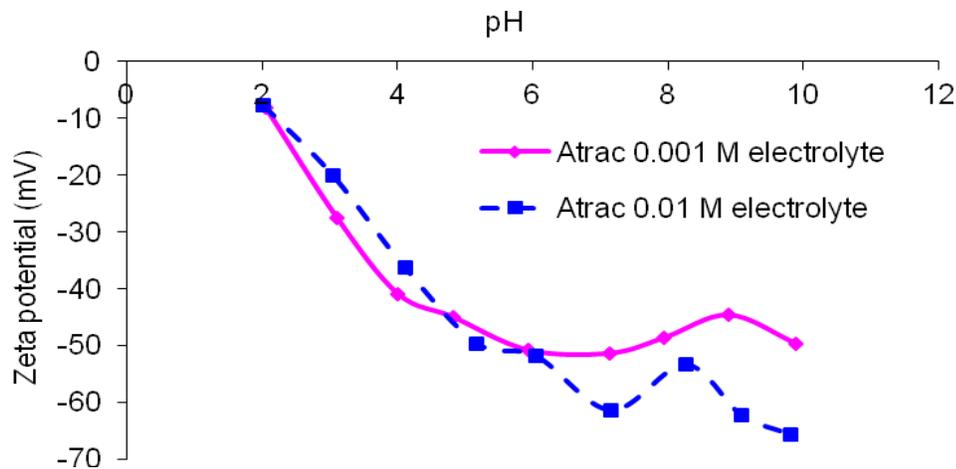
Fig. (5). Zeta-potential versus pH of collector colloidal species at 0.01 and 0.001 M ionic strength.
