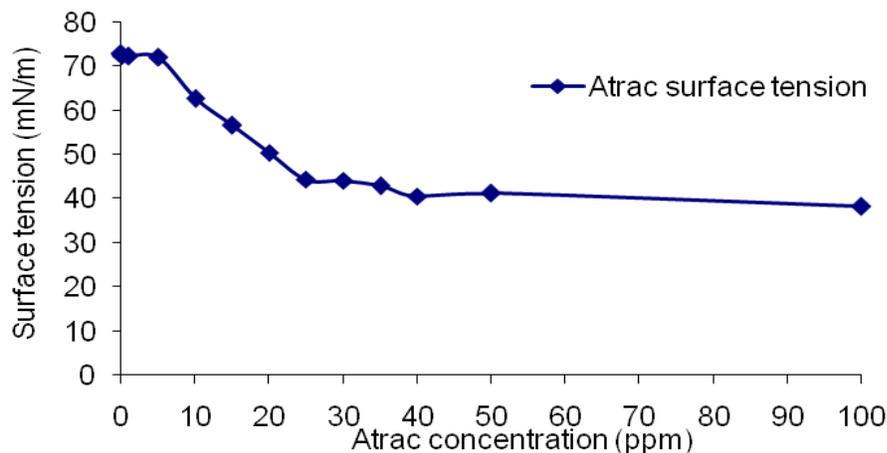
Fig. (2). Surface tension of aqueous solution of Atrac collector at pH 8.5.
