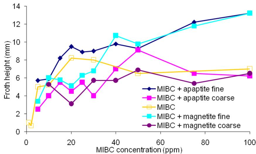
**Fig. (16).** Froth formation in the presence of apatite and magnetite particles as a function of frother concentration.
