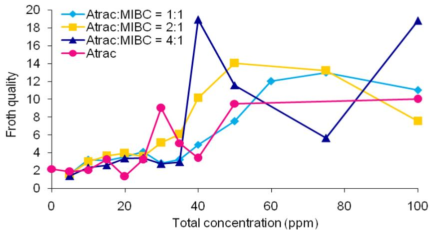
Fig. (13). Froth quality at different collector and frother composition as a function of total concentration at pH 8.5.
