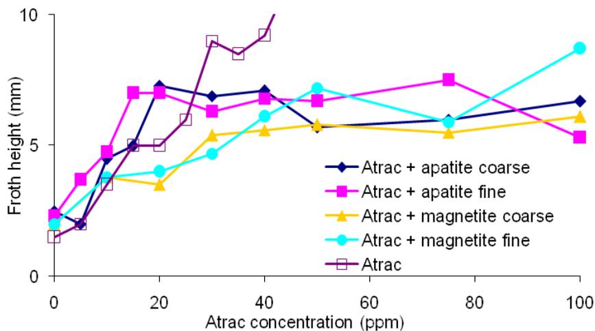
Fig. (14). Froth formation in the presence of apatite and magnetite particles as a function of collector concentration.
