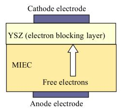
Fig. (2). Measuring the ionic activation energy of MIEC from the OCV.
