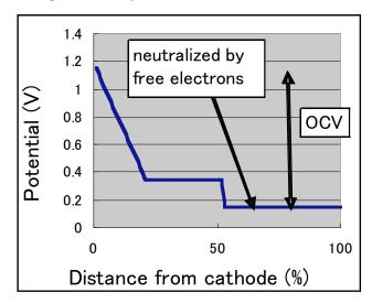
**Fig. (4).** Higher OCV values are obtained using small Ea, MIEC passivation films.
