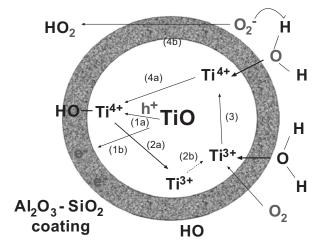
Fig. (4). Surface photocatalytic activity of Titanium Dioxide.
