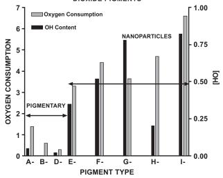
Fig. (5). Comparison of hydroxyl content and oxygen consumption rates for 2-propanol oxidation with pigmentary and nano particle titanium dioxide.
