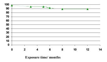
**Fig. (28).** Percentage efficacy of NOX reduction for a typical silicate paint film with weathering.
