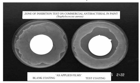
Fig. (13). A typical anti-bacterial evaluation on an agar plate medium for eco-paint films with and without nanoparticluate photocatalyst titania.
