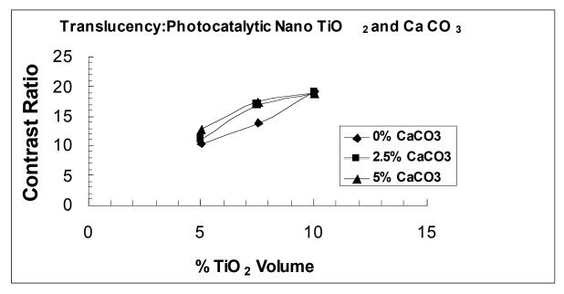
Fig. (27). Translucency (contrast ratio) for BS 45 paint films with volume addition of sol-gel anatase titania (10-20 nm) particles versus % calcium carbonate addition.
