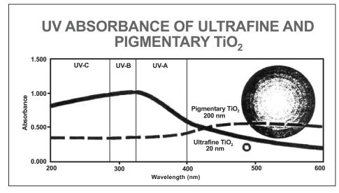
Fig. (2). Comparison of the optical behaviour of ultrafine TiO<sub>2</sub> and pigmentary TiO<sub>2</sub>.
