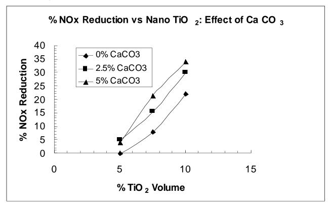
**Fig. (25).** Percentage NOx reduction versus volume of titania (anatase 10-20 nm) for a polysiloxane BS45 paint substrate with 0, 2.5 and 5.0% w/w of nanoparticle calcium carbonate.
