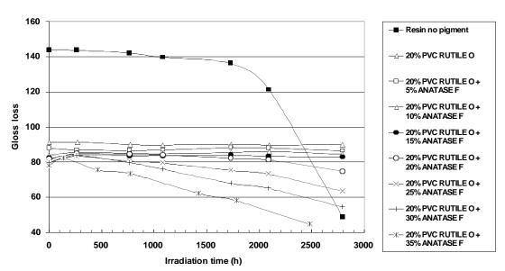
**Fig. (10).** Gloss loss versus irradiation time in a QUV weatherometer for a DSM siliconised polyester resin with 20% w/w Rutile pigment O plus increasing levels of 5, 10, 15, 20, 25, 30 and 35 % w/w of nanoparticle anatase F.
