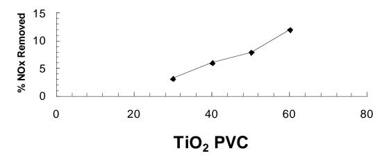
Fig. (24). Percentage concentration of NOx removed versus the concentration of anatase sol-gel particles (10-20 nm) at 5% w/w in a polysiloxane Wacker BS 45 paint system.
