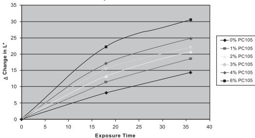
Fig. (9). Change in colour difference factor L with exposure time for metylene blue impregnated silicate paint films with increasing nanoparticle titanium dioxide PC-105.
