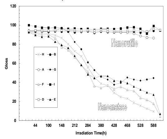
Fig. (6). Loss of gloss during weathering of an alkyd Paint film in an Atlas weatherometer.
