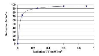
**Fig. (29).** Reduction in NOx with Radiation Uv intensity for a typical Eco-silicate paint film.
