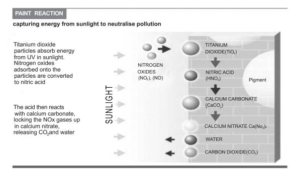
Fig. (21). Depollution scheme for photocatalytic paints and surfaces.
