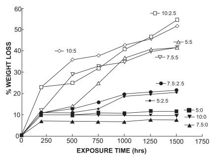
Fig. (26). Percentage weight loss versus exposure time in an Atlas Ci65 weatherometer for polysiloxane paint films (BS 45) containing different ratios of nano anatase (10-20 nm) sol-gel titania (5/7.5/10):calcium carbonate (0/2.5/10)particles.
